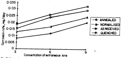
Fig.7: Corrosion rate with Concentration of extraneous ions at %0.6 Fe content.
