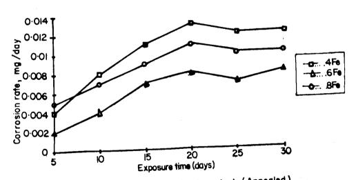
Fig.2. Corrosion rate with exposure time at % Fe content, (Annealed)
