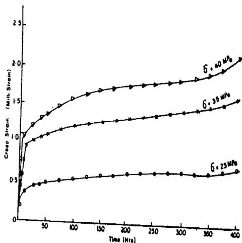
Fig. 2: GRP Creep Experimental Response
