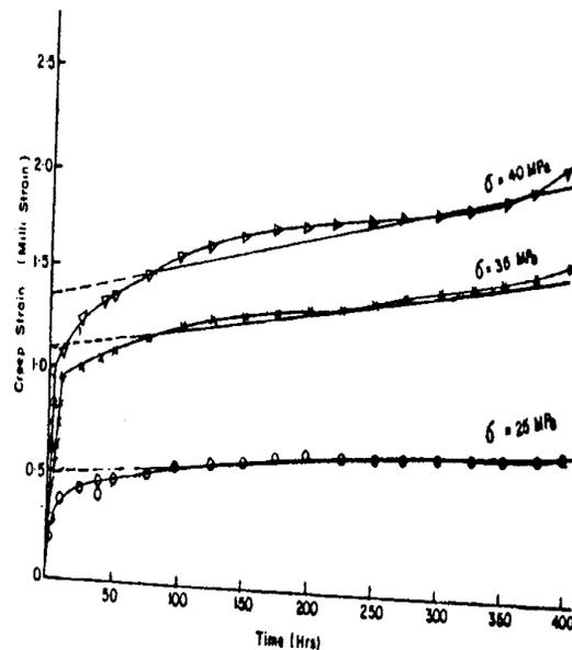
Fig. 3: Empirical Steady Creep Strain Rates Fitted on Experimental Curves
