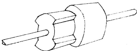
Fig. 1: The composite magnetic rotor structure
