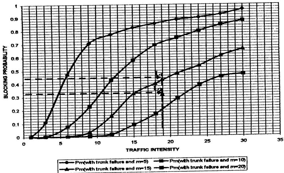
Figure 8: Blocking probability vs traffic intensity for varied numbers of trunk lines with failure.
