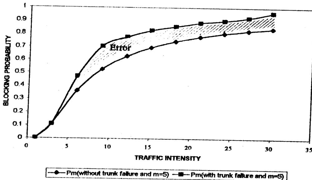
Figure 4: Blocking probability vs traffic intensity for  $m=5$ ;  $\alpha=1.157E-5$ ;  $\beta=5.787E-6$
