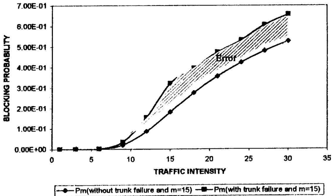
Figure 6: Blocking probability vs traffic intensity for  $m=15$ ;  $\alpha=3.472E-5$ ;  $\beta=1.736E-5$
