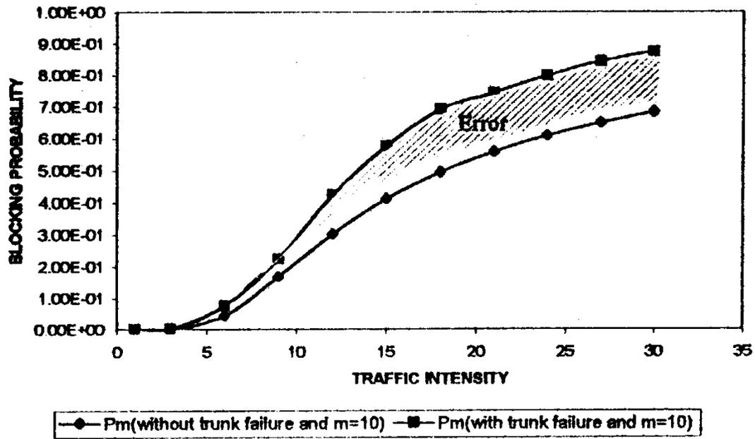
Figure 5: Blocking probability vs traffic intensity for  $m=10$ ;  $\alpha=2.315E-5$ ;  $\beta=1.157E-5$
