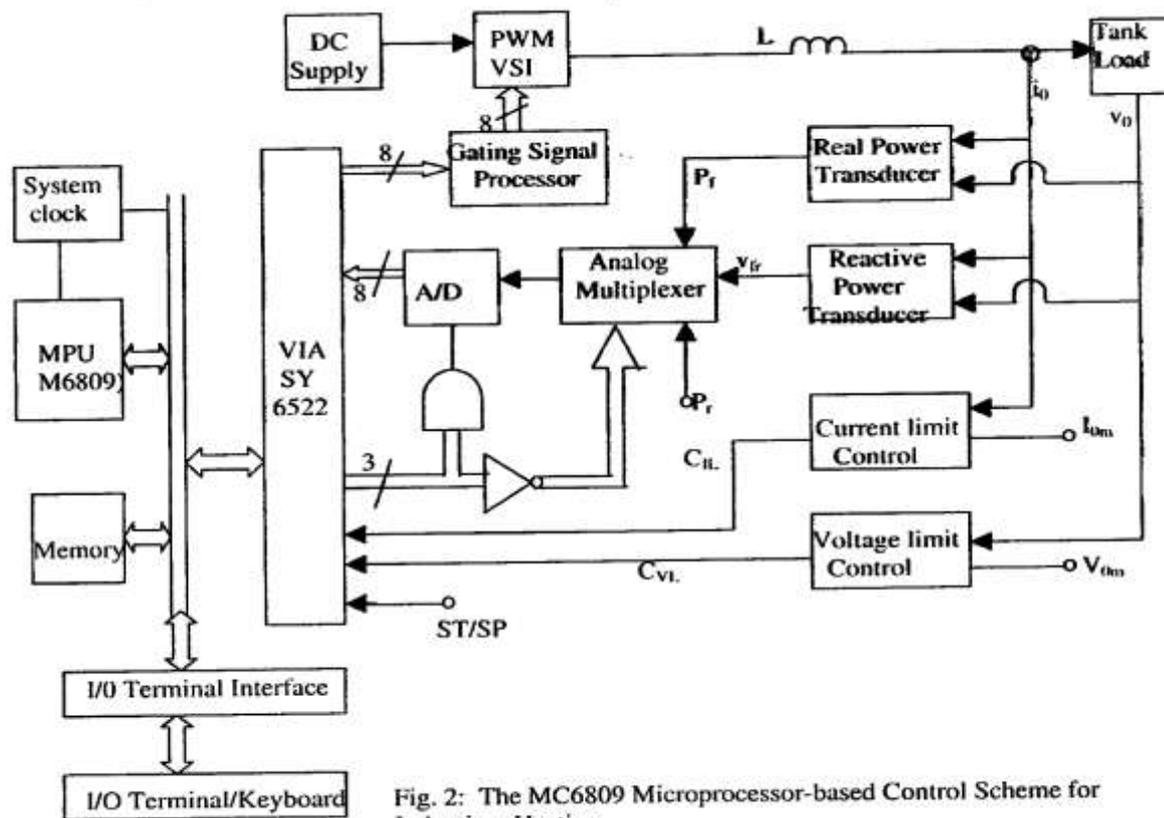
Fig. 2: The MC6809 Microprocessor-based Control Scheme for Induction Heating
