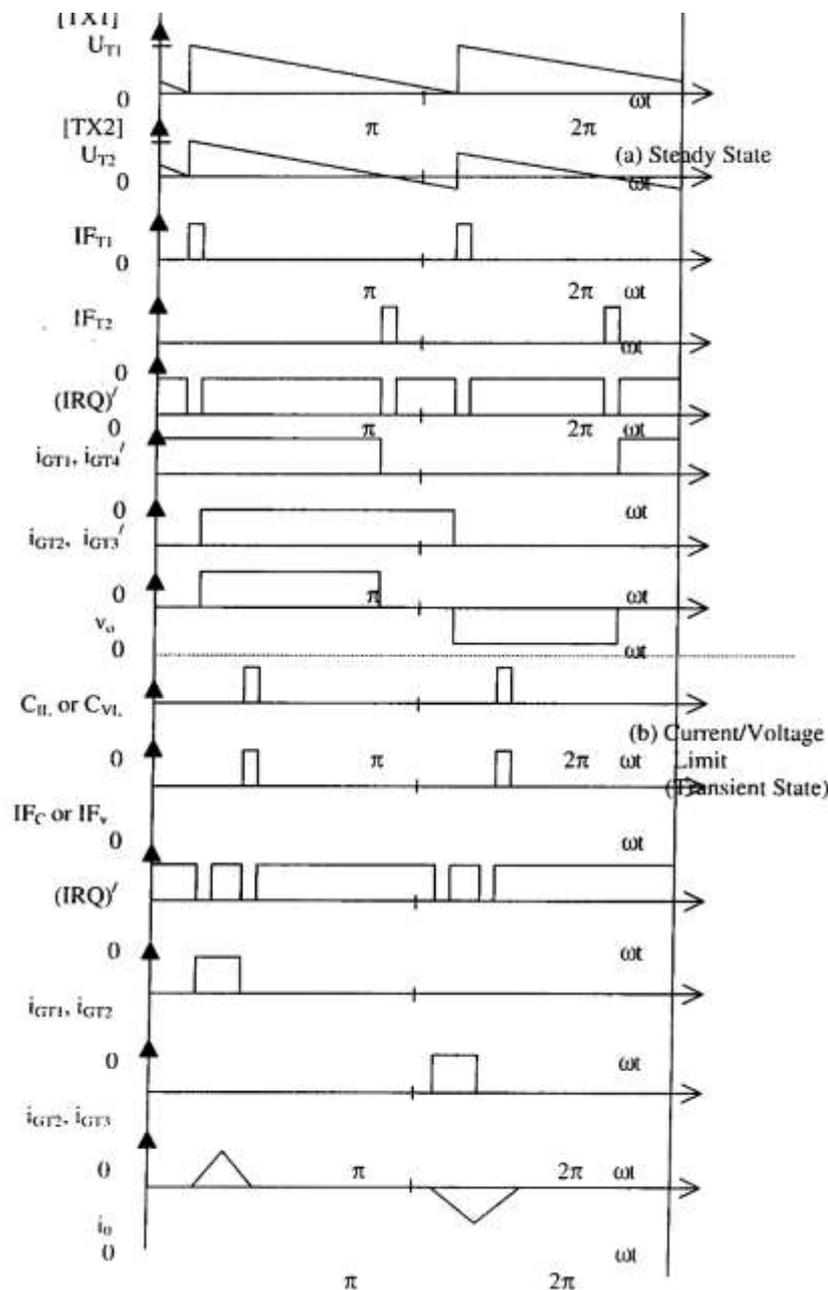
Microprocessor-based Gating Signal Generation for the Dual Modulation Method
