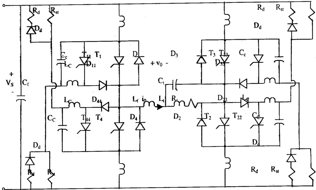
Fig. 1: The PWM Single Phase Voltage Source Inverter with an Induction Heating Tank Load.
