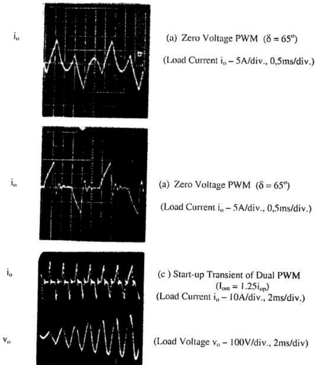
Fig. 4: Experimental Steady State and Start-up Transient waveforms of the Inverter with a Tank Load ( $V_s=189V, X_{Lto} = 6.8\Omega, Z_{to} = 34 \Omega, C_t = 130\mu F$ )
