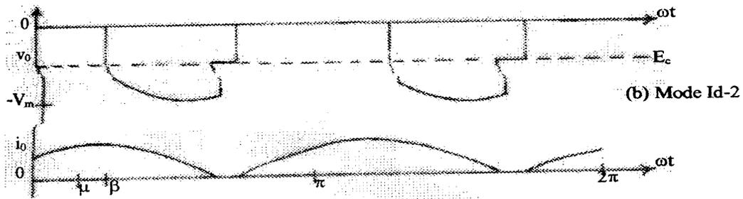
Fig. 6: Load Current ( $I_{c-2}$  &  $I_{d-2}$ ) in the Range  $\mu \leq \beta \leq \pi/2$
