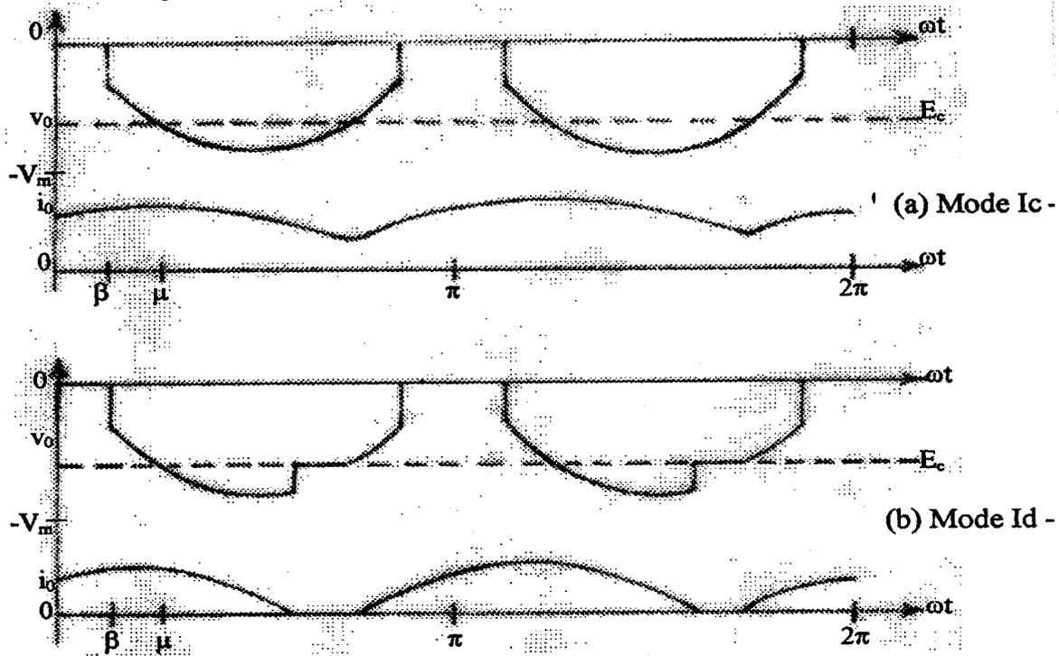
Fig. 5: Load Current Modes in the Range of  $0 < \beta < \mu$  (Inversion).
