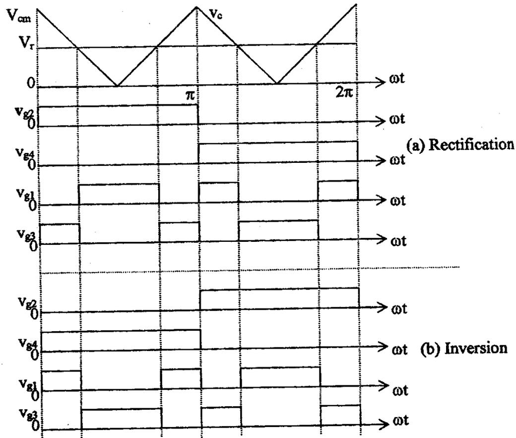
Fig. 2: PWM Gating Signals for the AC/DC Converter of Fig. 1.
