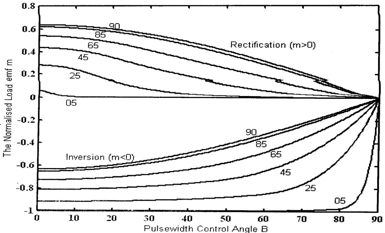
Fig. 7: The p.u. Boundary Load emf  $m$  Versus Switching Angle  $\beta$ .
