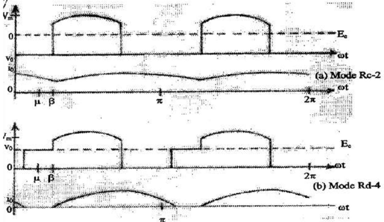
Fig. 4: Load Current Modes in the Range of  $\mu \leq \beta \leq \pi/2$  (Rectification).
