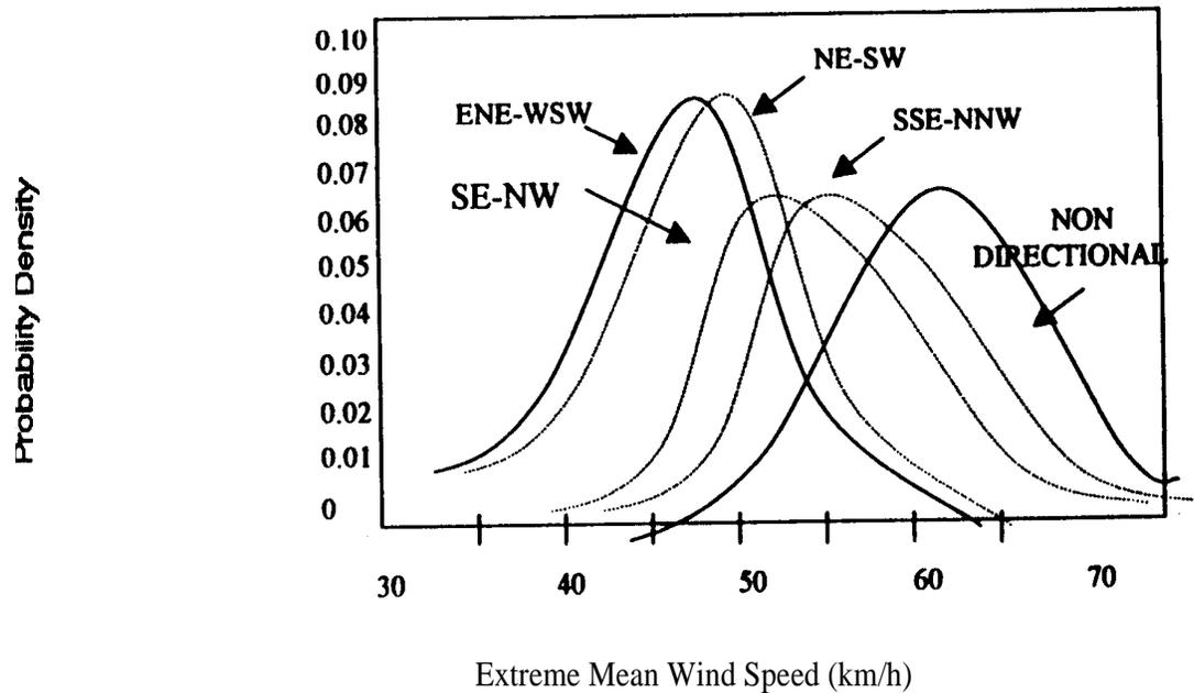
Fig.4 probability Density Functions of the Extreme Winds Speeds for typical line orientations
