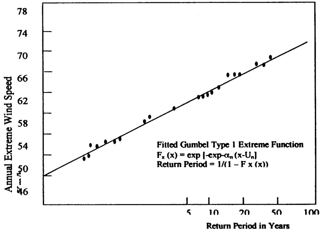
Fig. 2 Set of Annual Extreme Wind Speeds in NE-SW Direction fitted by Type 1 Asymptotic Extreme Value Distribution
