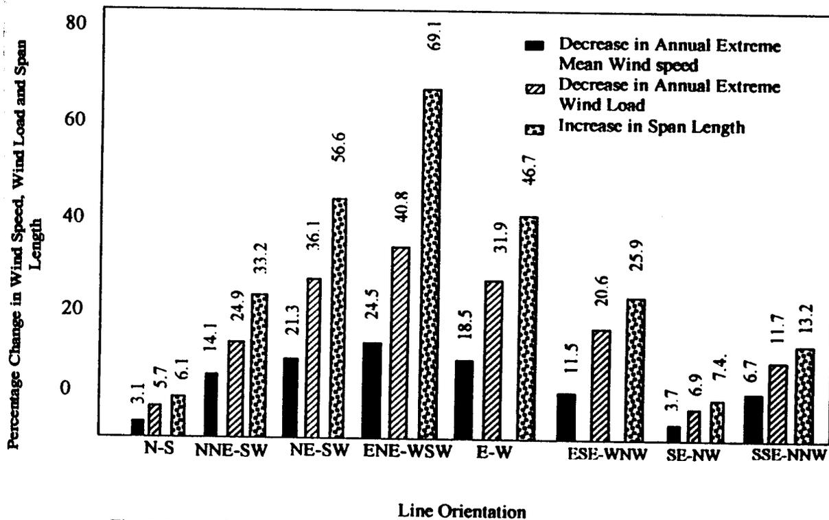
Fig. 7 Change in Annual Extreme Wind Speed, Wind Load, and Span Length for Different Line Orientations
