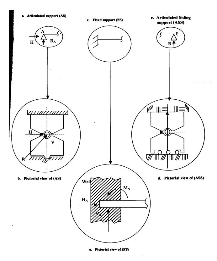
Fig.2. non -deformable rigid supports
