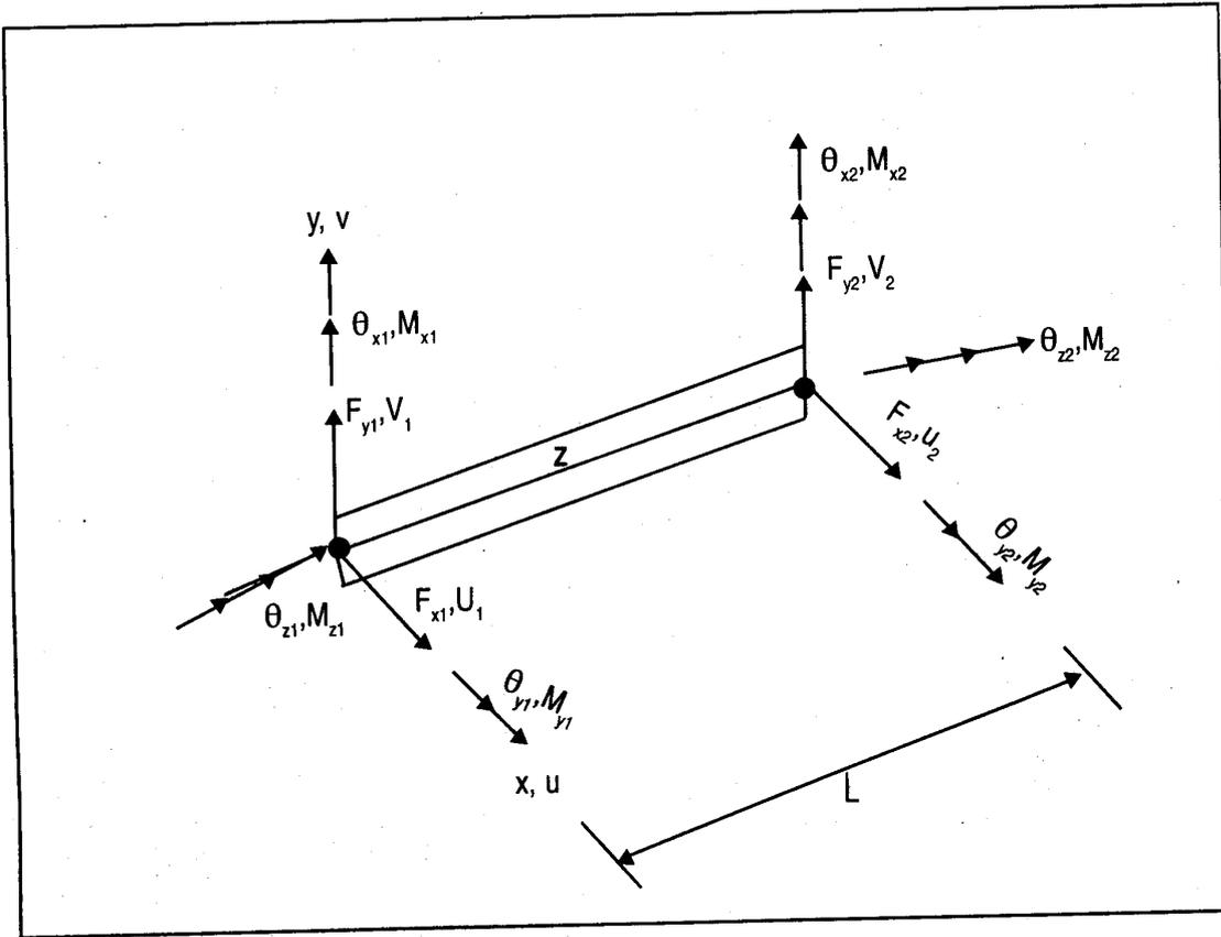
Fig. 1: Prismatic beam element for present Formulation.
