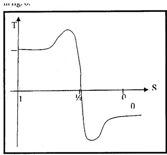
Fig. 6: Torque-slip curve of the machine
