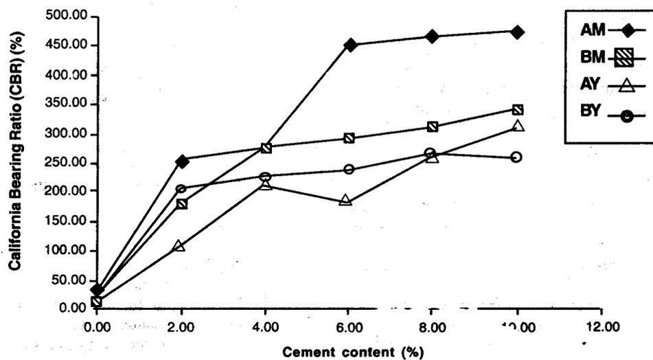
Fig. 4: Variation of California Bearing Ratio with Cement content.
