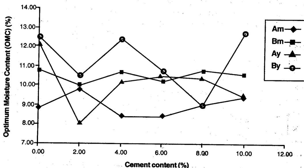
Fig. 2: Variation of Optimum Moisture Content with Cement content.
