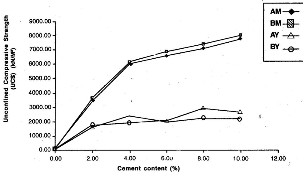
Fig. 3: Variation of Unconfined Compressive Strength with Cement content.
