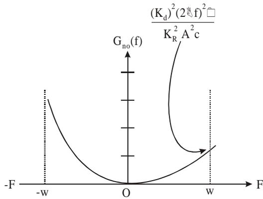
Fig .2 shows Noise Power Spectrum in FM Systems.
