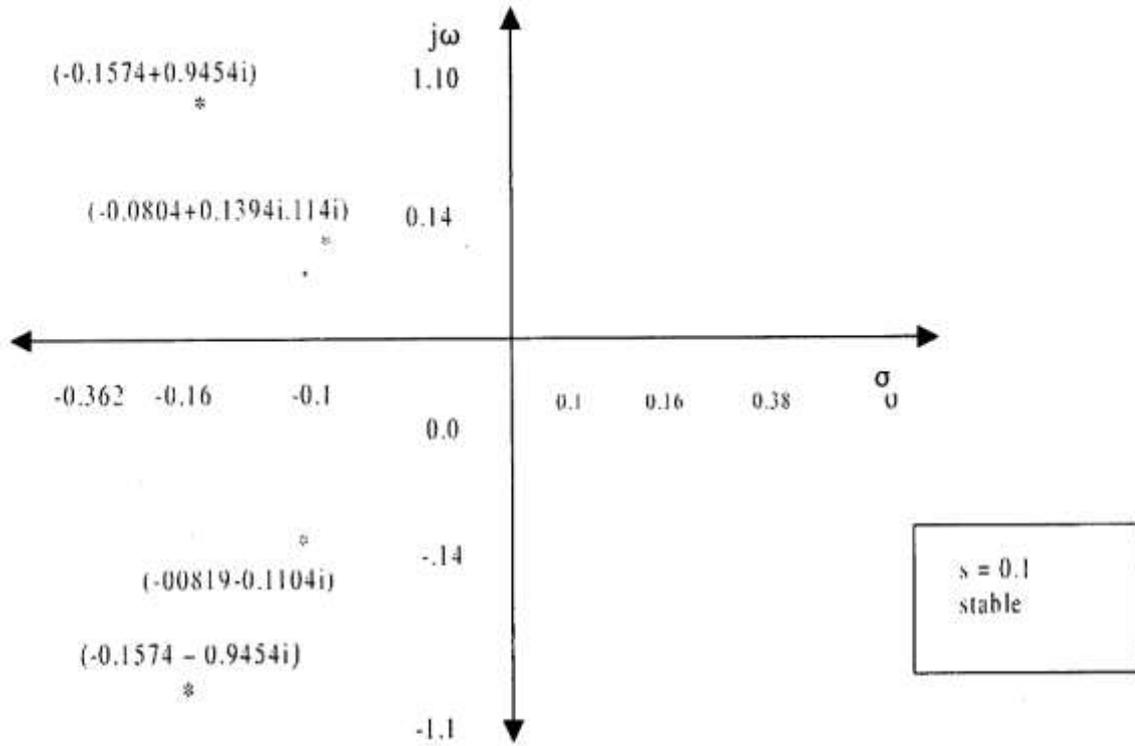
Fig. 2: Polar plot for slip = 0.1.
