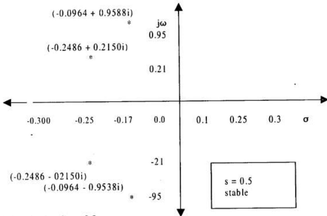
Fig. 6: Polar plot for slip = 0.5.
