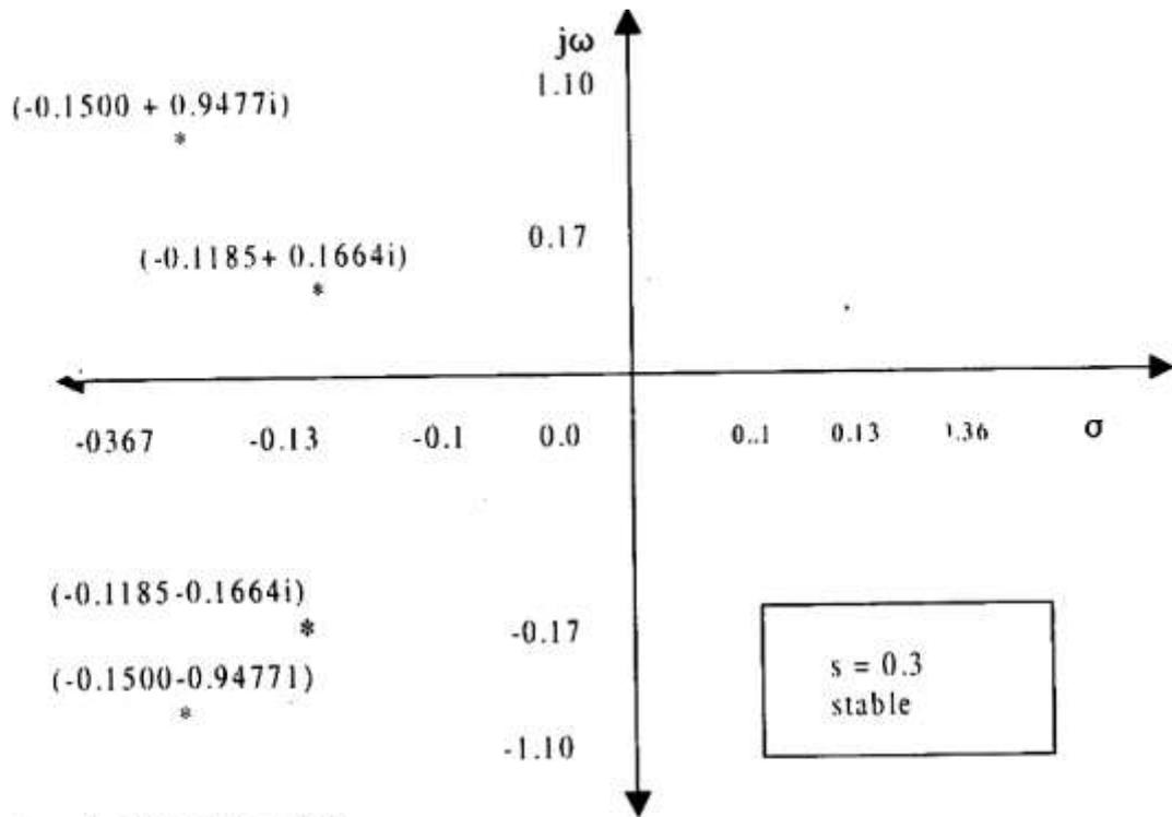
Fig. 4: Polar plot for slip = 0.3.
