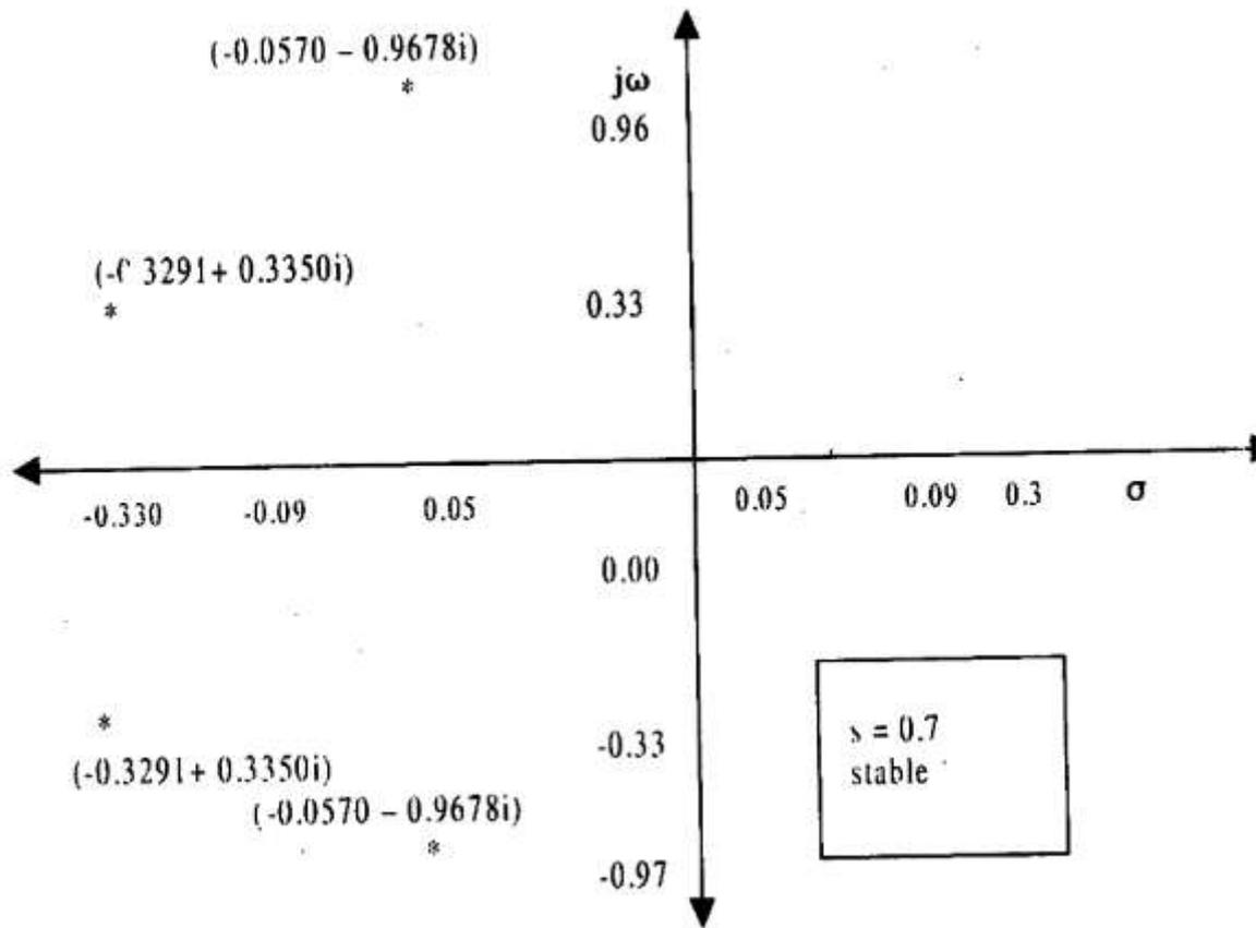
Fig. 8: Polar plot for slip = 0.7
