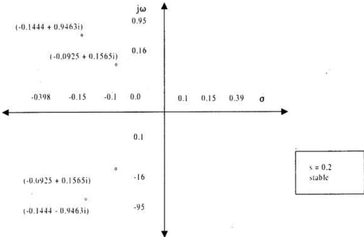
Fig. 3: Polar plot for slip = 0.2.
