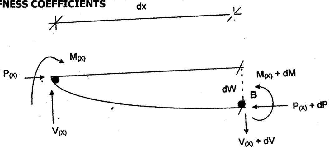
**Fig. 1: A section of a Beam-Colum**
