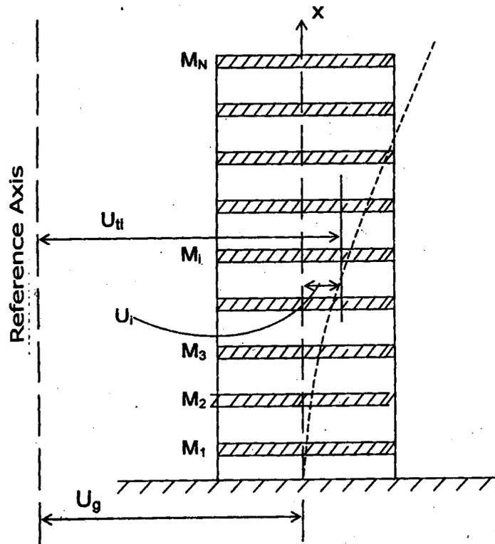
Fig. 1: Lumped MDOF System with Rigid Base Translation
