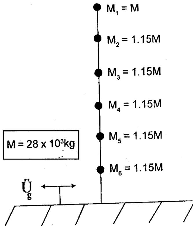
**Fig. 3** A 6-DOF System subject to ground motion.
