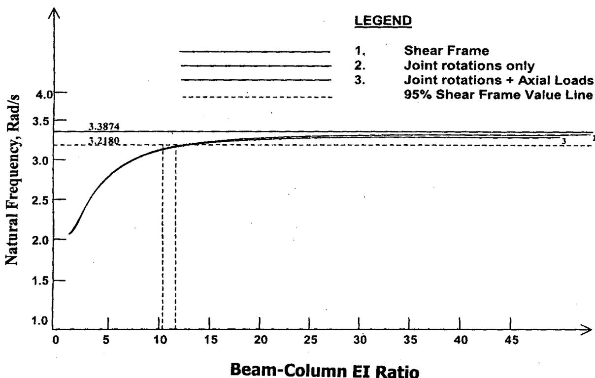
**Fig 4:** Plot of Natural Frequency Against Beam-Column EI Ratio for the 15-Storey Frame.
