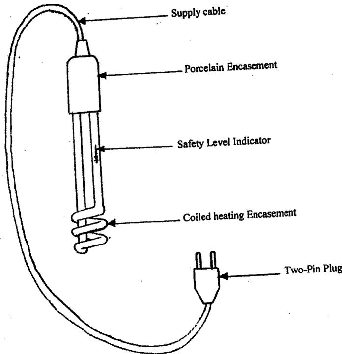
Fig.1: Heater without control Unit
