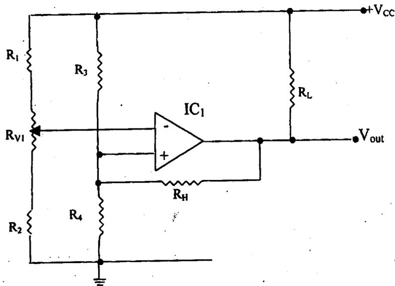
**Fig.5:** The Schmitt trigger
