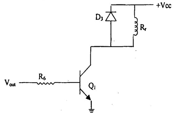
Fig. 7: Relay Driver network.
