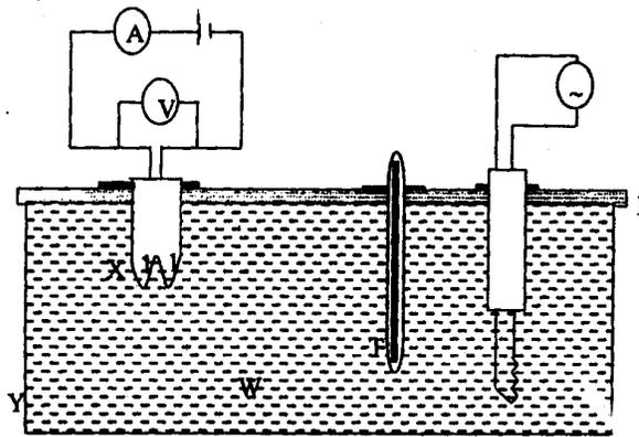
**Fig.4** Scheme for measurement of Conductance of water
