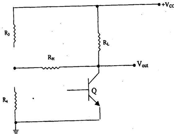
Fig. 6: Equivalent circuit of the Schmitt trigger
