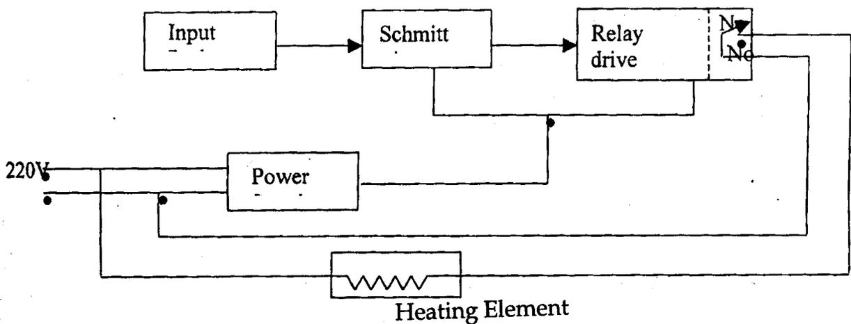
Fig. 2 Block diagram of the Control unit.
