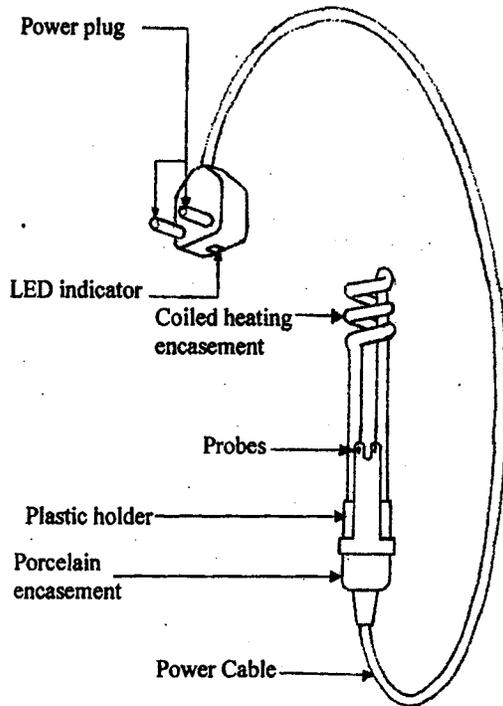
*Fig 8. Water heater with safety control unit.*
