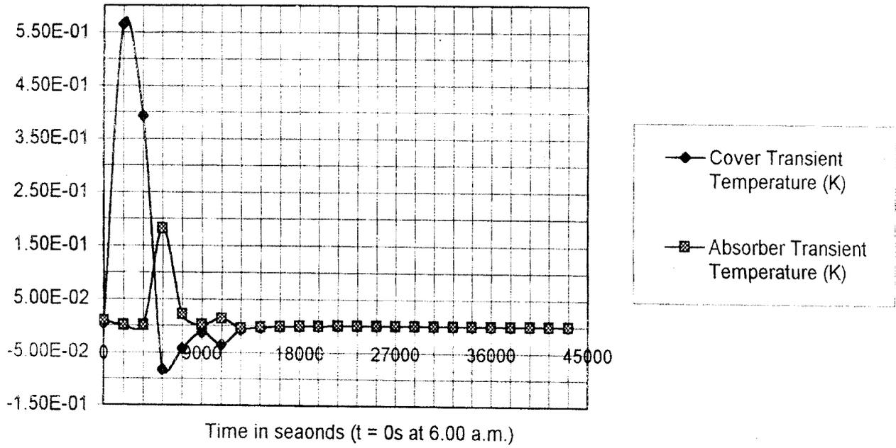
Fig. 7a SSSCA Flat Plate Collector Model Plates' Transient Temperatures on 21-03-02
