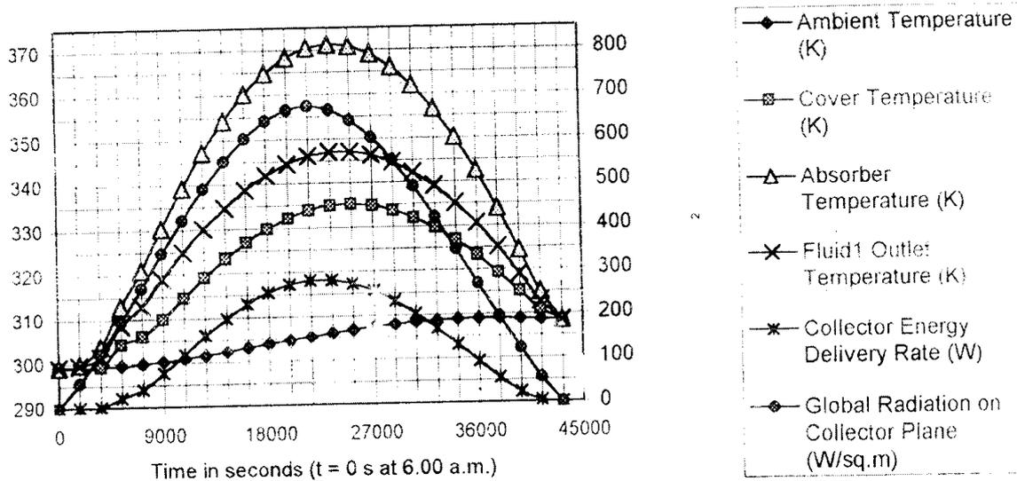
Fig 2a SSSCA Flat Plate Collector Model Input and Output Parameters on 14-03-02
