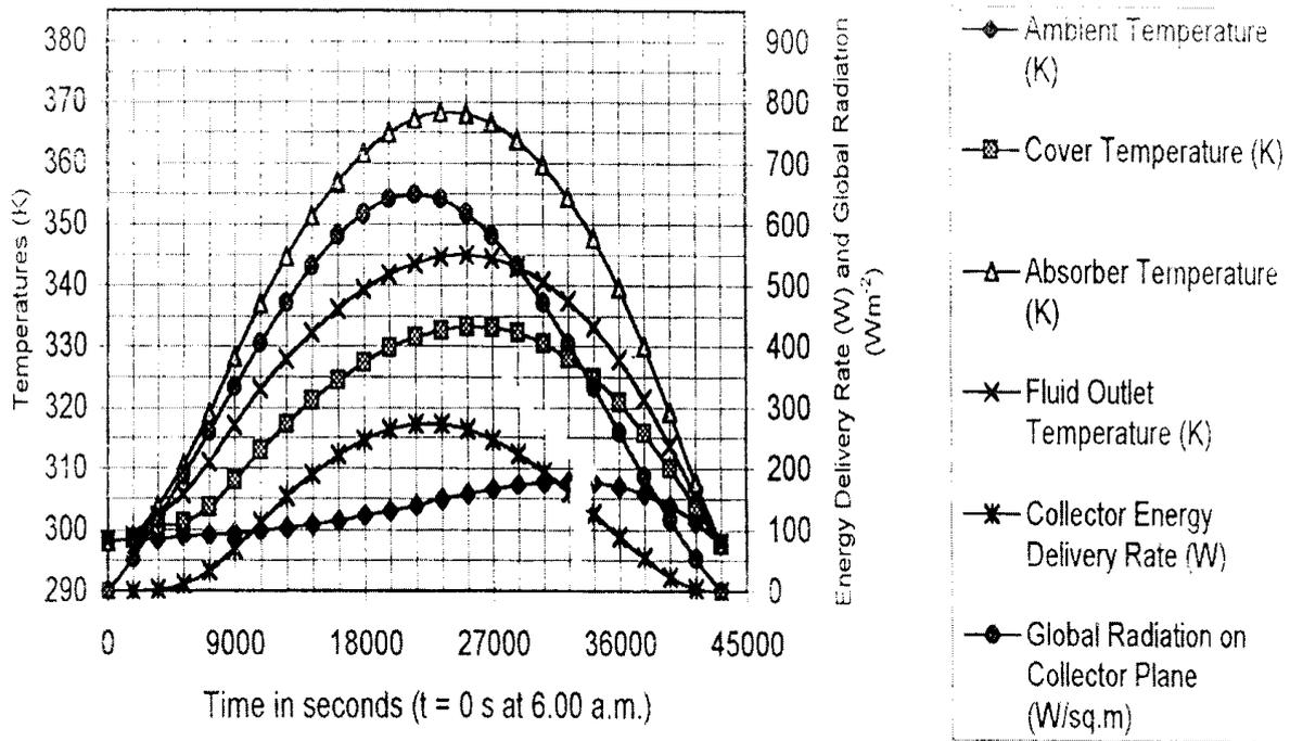
Fig. 3a SSSCA Flat Plate Collector Model Input and Output Parameters on 16-03-02
