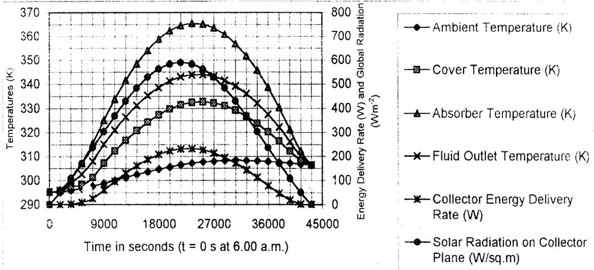
Fig 4a SSSCA Flat Plate Solar Collector Input and Output Parameters on 21-03-02
