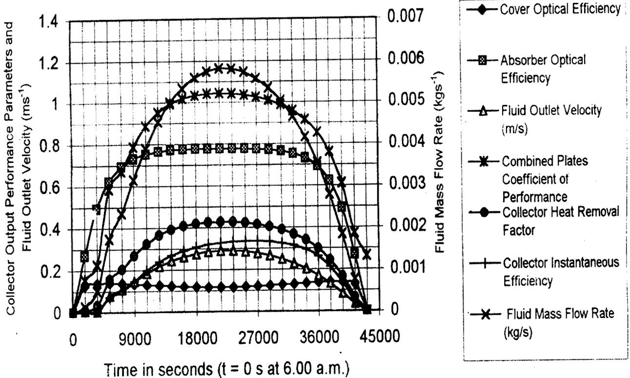
Fig. 5b SSSCA Flat Plate Collector Model Output Performance Parameters and Fluid Mass Flow Rate and Outlet Velocity on 23-03-02
