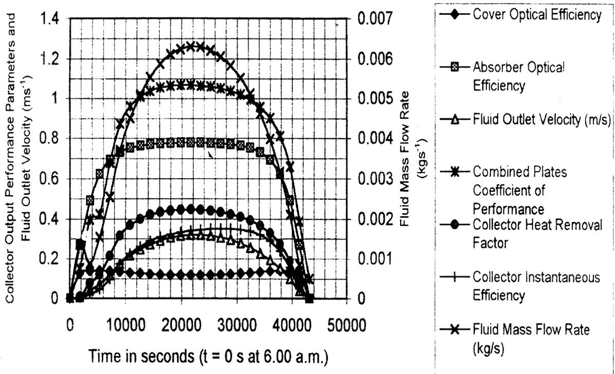
Fig. 4b. SSSCA Flat Plate Collector Model Output Performance Parameters and Fluid Mass Flow Rate and Outlet Velocity on 21-03-02
