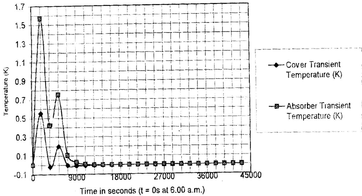
Fig. 7b SSSCA Flat Plate Collector Model Plates' Transient Temperatures on 23-03-02
