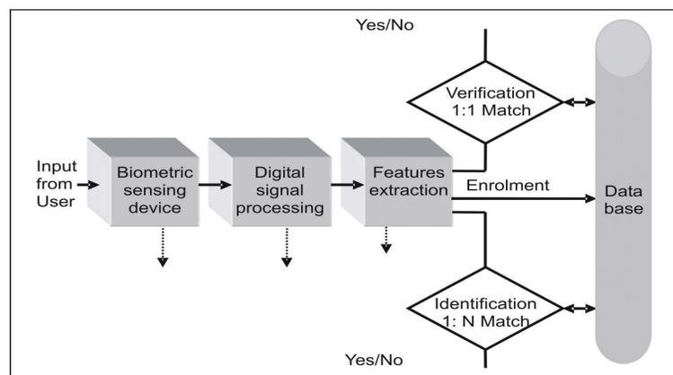
Fig 1: Diagram of Automated Biometric Systems
