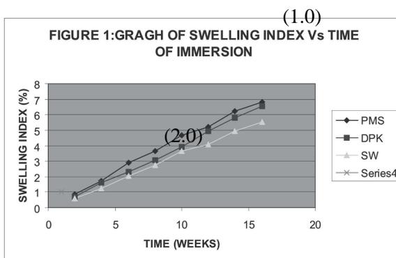
organic liquids penetrate and swell the polymeric composite through diffusion and absorption phenomena. Hence allowing crazing (formation of micro voids) to take place at lower stresses and once a craze has formed; the active environment is able to diffuse along the craze more easily than through the bulk material.
