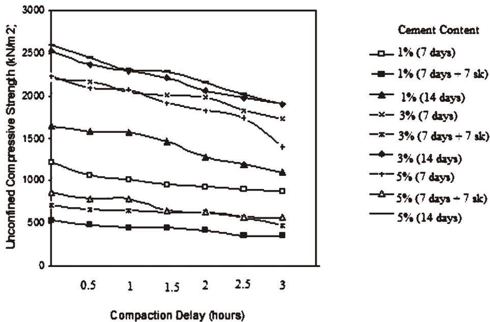
**Figure 4: variation of Unconfined Compressive Strength with Compaction Delay for Red lateritic soil**
