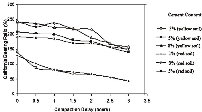
**Figure 5: Variation of California Bearing Ratio with Compaction Delay for stabilized lateritic soils**
