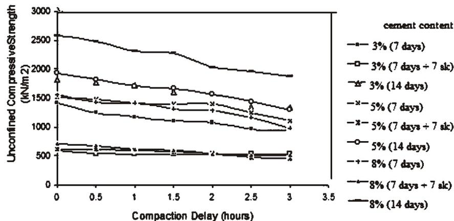
**Figure 3: Variation of Unconfined Compressive Strength with Compaction Delay for Yellow lateritic soil**
