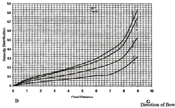
Fig 10: Comparison of Velocity Distribution Across Canal Entrance for Different Ratios of Canal and Channel Widths
