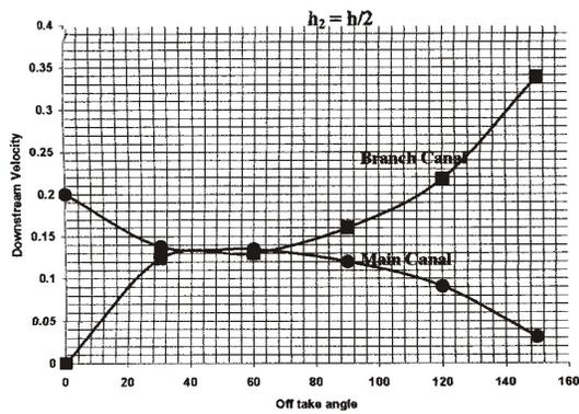
Fig 12: Comparison of Downstream Velocities of Canal and Channel for Different Off Take Angles ( $h_2 = h/2$ )
