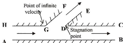
Fig 8: Channel with Branch Canal Showing Critical Points the downstream end (point D) is a stagnation
