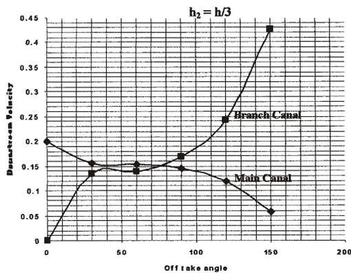
Fig 14: Comparison of Downstream Velocities of Canal and Channel for Different off Take Angles ( $h_2 = h/3$ )
