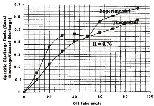
Fig 15: Specific Discharge Ratio Versus Off Take Angle for  $Q = 0.196 \text{ m}^3/\text{s}$
