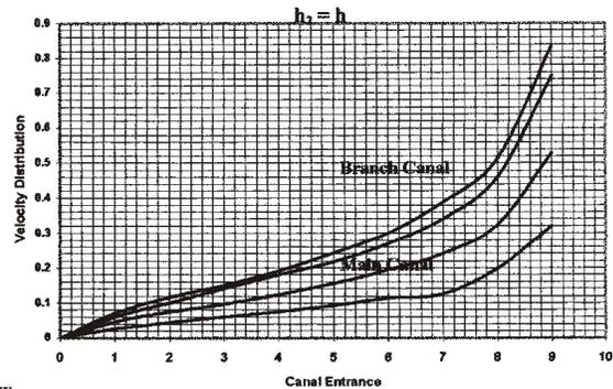
Fig 11: Comparison of Downstream Velocities of Canal and Channel for Different Off Take Angles ( $h_2 = h$ )
