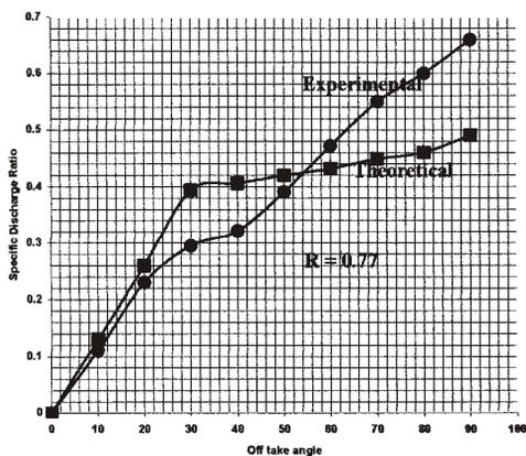
Fig 16: Specific Discharge Ratio Versus Off Take Angle for  $Q = 0.126 \text{ m}^3/\text{s}$
