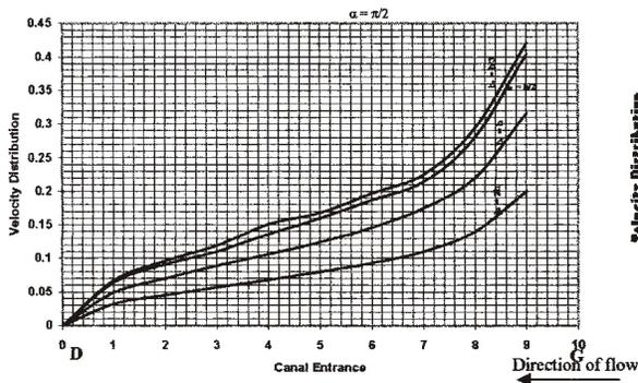
Fig 8: Comparison of Velocity Distribution Across Canal Entrance for Different Ratios of Canal and Channel Widths
