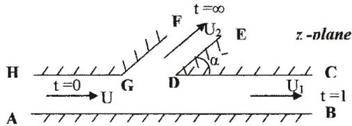
Fig 4: Channel with a Branch Canal Taking of at Angle  $\alpha$
