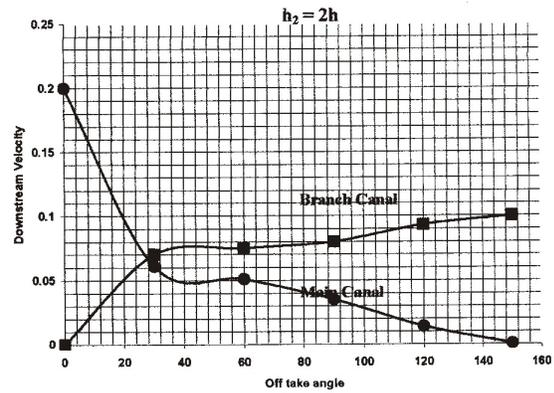
Fig 13: Comparison of Downstream Velocities of Canal and Channel for Different Off Take Angles ( $h_2 = 2h$ )
