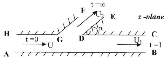
Fig 2: Channel with a Branch Canal Taking off at Angle  $\alpha$
