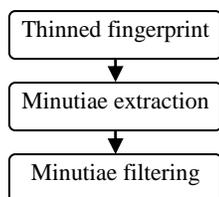
Figure 9: The stages of minutiae-based feature extraction of a fingerprint
