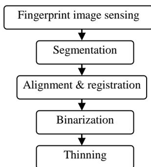
Figure 6: The stages involved in the image processing of a fingerprint.
