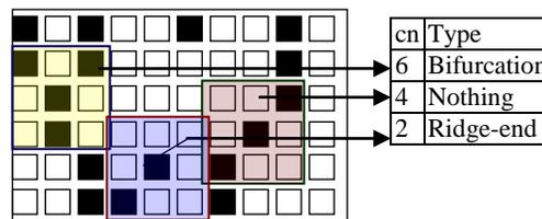
Figure 10: Detection of minutiae types using the crossing number technique
