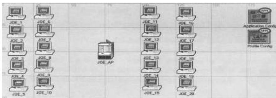
Figure 3: A view of the network in a scenario with 20 stations and one access point
