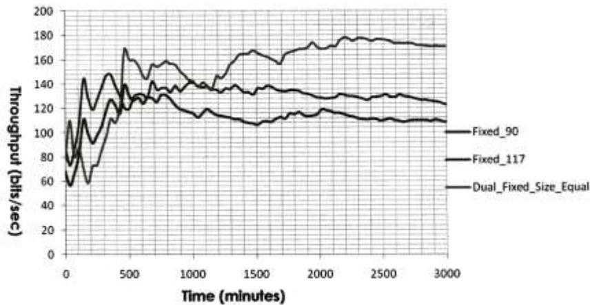
Figure 5: Dual fixed case with equal proportion of 90 and 117 bytes frames
