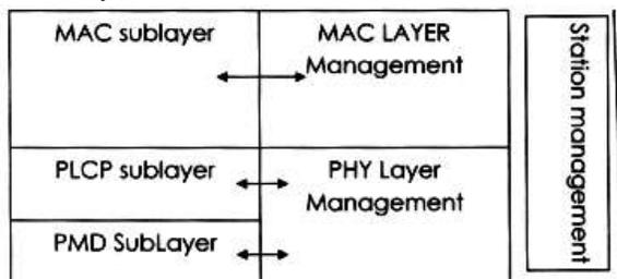
Figure 1: OSI model for IEEE 802.11 (MAC layer is the Data link layer)
