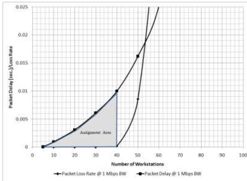
Figure 7. Packet delay/loss rate vs Number of workstations
