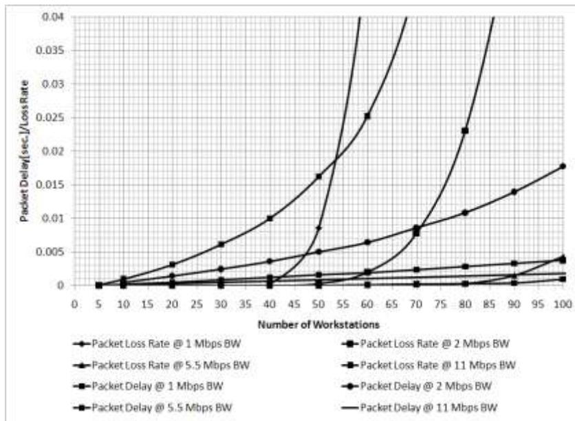
Figure 6. Packet delay/loss rate vs Number of workstations
