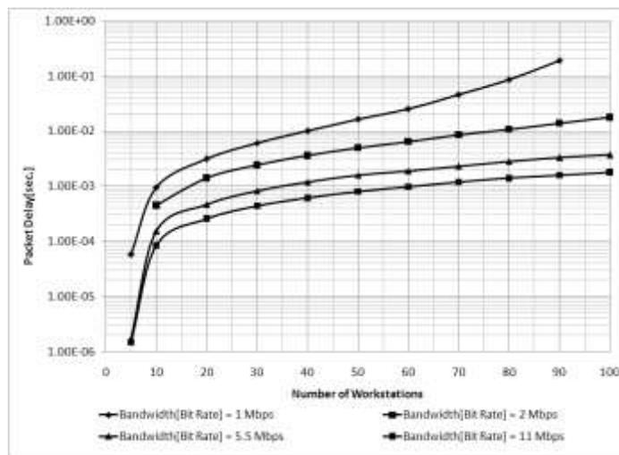
Figure 5. Packet delay vs Number of workstations (Buffer capacity = 50[packets])
