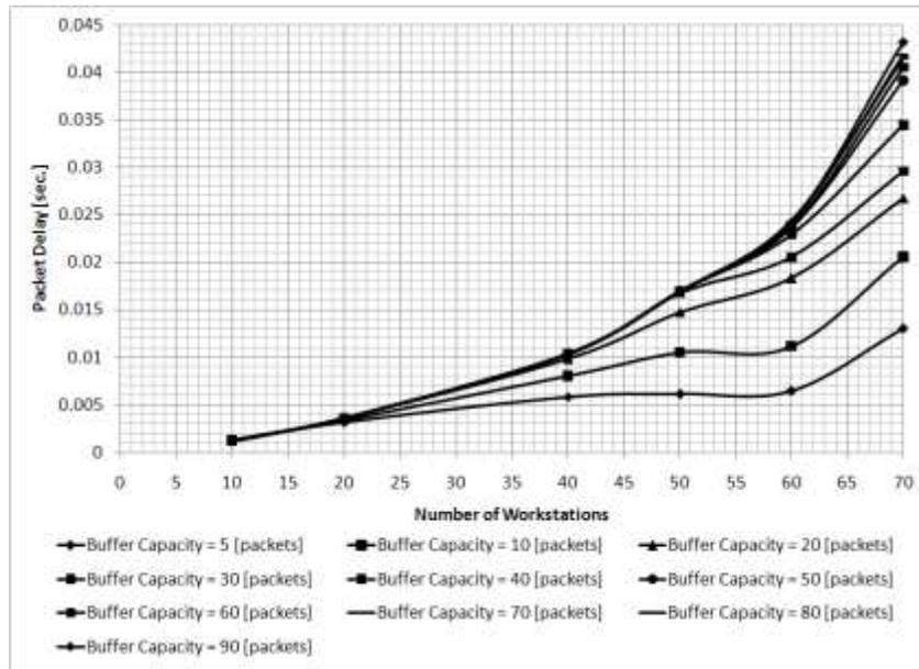
Figure 9. Delay vs Number of workstations (Transmission rate = 1Mbps)
