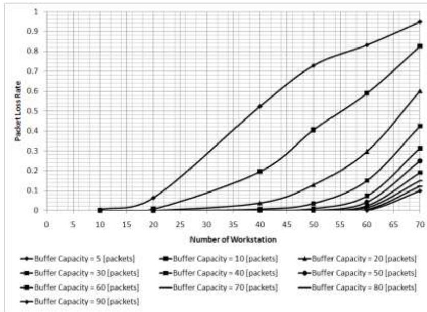
Figure 8. Packet loss rate vs Number of workstations (Transmission rate = 1Mbps)
