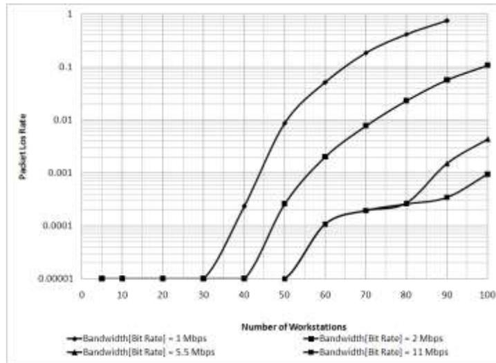
Figure 4. Packet loss rate vs Number of workstations (Buffer capacity = 50 [packets])
