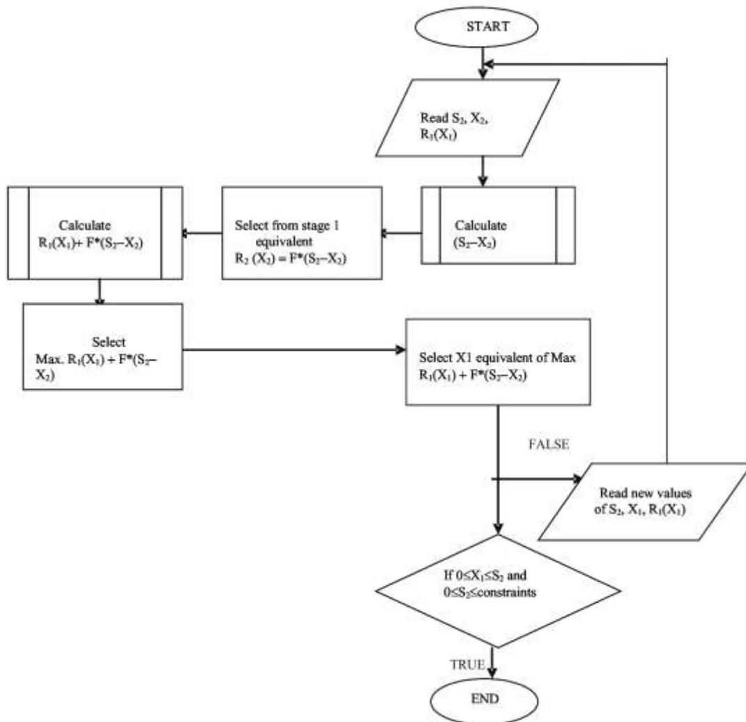
Fig3: The Algorithm of Stage 2 Flowchart of the TORA Software Dynamic Programming Calculations.
