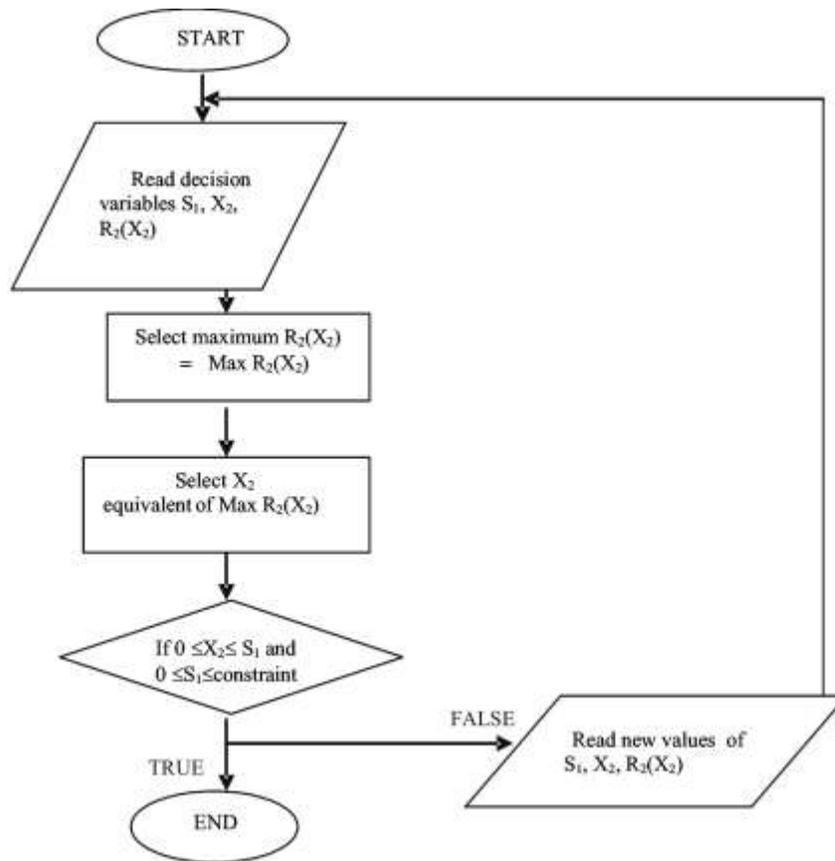
Fig 2: The Algorithm of the Stage 1 Flowchart of the TORA Software Dynamic Programming Calculations.
