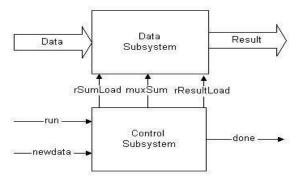
Figure 6: View of Data and Control subsystems
