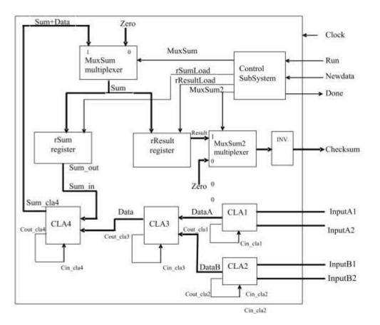
Figure 7: Modified Checksum System
