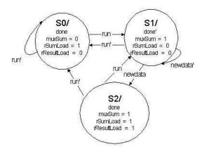
Figure 4(b): Multiplexer/Register-level
