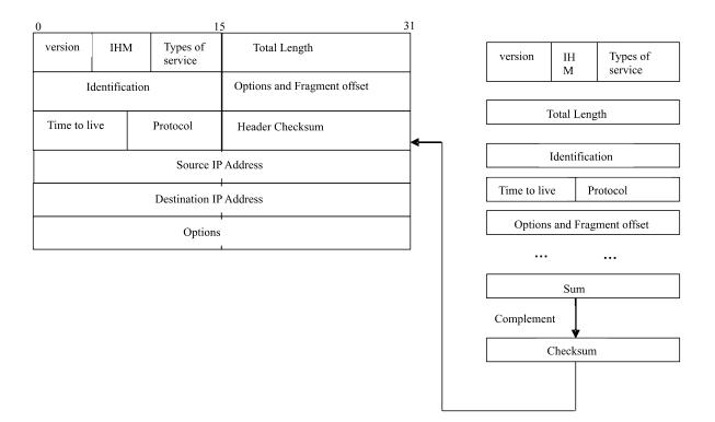
Figure 1: Checksum Calculation for IP Packet Header
