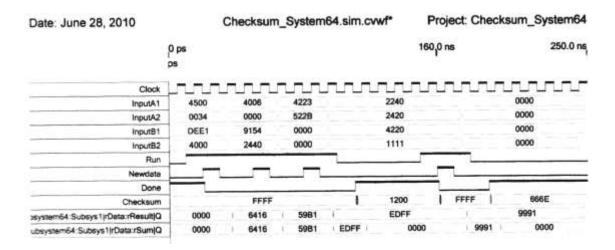
Figure 10: The waveform for the timing simulation
