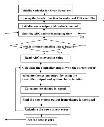
Figure 13: Flowchart for PID algorithm.
