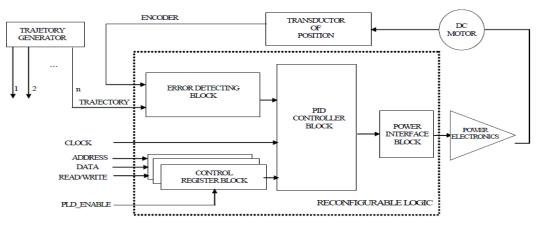
Figure 14: DMC system control blocks.
