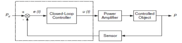
Figure 5: Closed-loop speed control system
