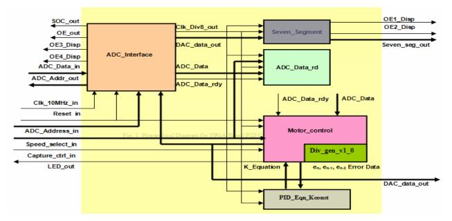
Figure 17: PID Controller Top module with sub modules.
