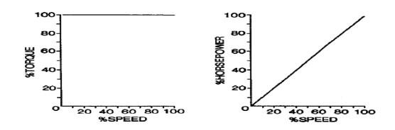
Figure 3: PM DCM Constant torque characteristics.
