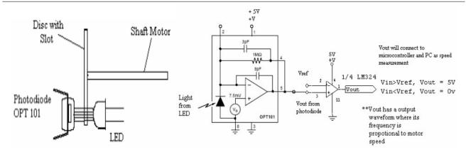
Figure 10: (a) Basic configuration (b) Schematic circuit.
