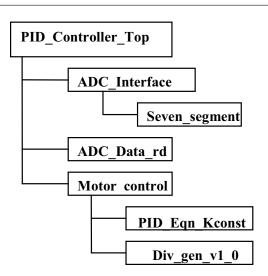
Figure 16: Hierarchical Diagram of PID controller Implementation.
