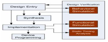
Figure 7: Programmable logic design methodology.
