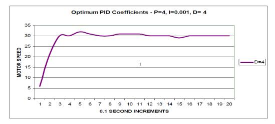
Figure 20: Experimental result of conventional PID control (motor speed scale = X 10 RPM).
