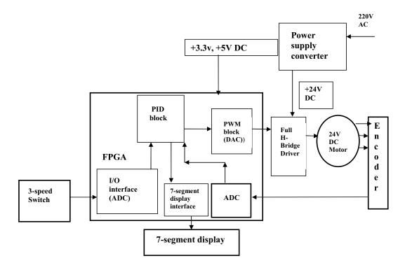
Figure 8: DMC Architecture and functional modules.
