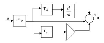
Figure 6: PID controller schematics.
