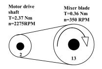
Figure 11: DCM drive shaft and Mixer agitator shaft and pulley system.
