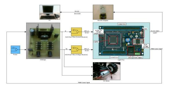
Figure 18: DMC - FPGA experimental setup. Courtesy: http://dev.emcelettronica.com/print/51811.
