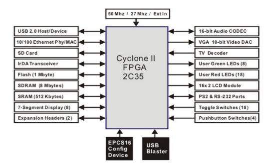
Figure 9: Altera DE2 FPGA development system.
