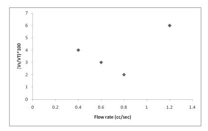
Figure 4: Percentage volume of sand in the produced fluid at different flow rate using light oil at confining pressure of 0MPa.
