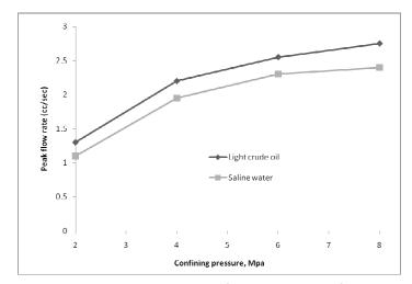
Figure 14: Relationship between peak flow rate and confining pressure.
