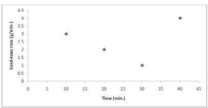
Figure 5: Mass flow rate of produced sand at different periods using light oil at confining pressure of 0 Mpa.
