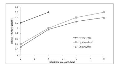
Figure 13: Relationship between critical flow rate and confining pressure.
