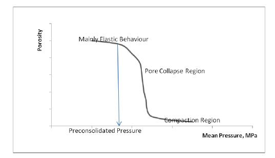
Figure 1: Porosity/stress curve showing elastic and pore-collapse regions.
