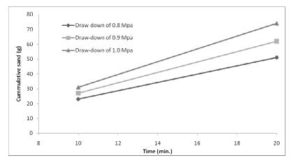
Figure 11: Cummulative sand produced at different draw-downs using light oil at confining pressure of 2 Mpa.
