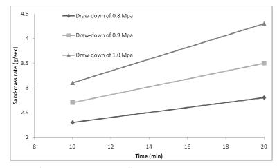
Figure 10: Mass flow rate of produced sand at different draw-downs using light oil at confining pressure of 2 Mpa.
