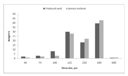
Figure 12: Grain size distribution of sand produced and porous medium at confining pressure of 2 MPa using light oil.
