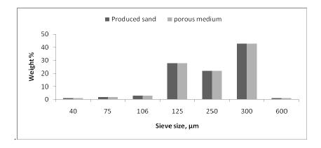
Figure 16: Grain size distribution of sand produced and porous medium at confining pressure of 2 MPa using heavy oil.
