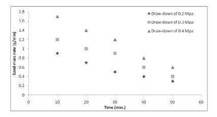
Figure 8: Mass flow rate of produced sand at different draw-downs using light oil at confining pressure of 2 Mpa.
