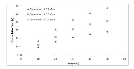
Figure 9: Cummulative sand produced at different draw-downs using light oil at confining pressure of 2 Mpa.
