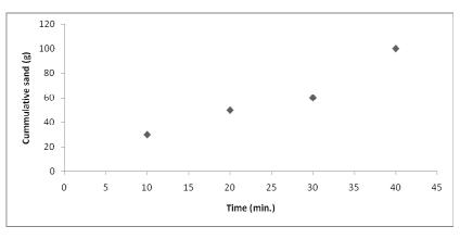
Figure 6: Cummulative sand produced at different time using light oil at confining pressure of 0 Mpa.
