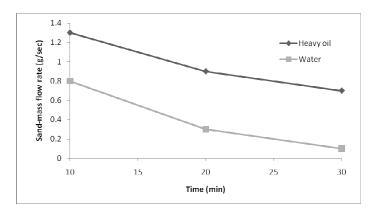
Figure 15: Mass flow rate of produced sand at different period using heavy oil at confining pressure of 2 Mpa.
