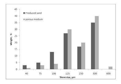
Figure 7: Grain size distribution of sand produced and porous medium at confining pressure of 0 MPa using light oil.
