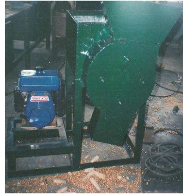
Figure 1: A pictorial view of the finished maize thresher.
