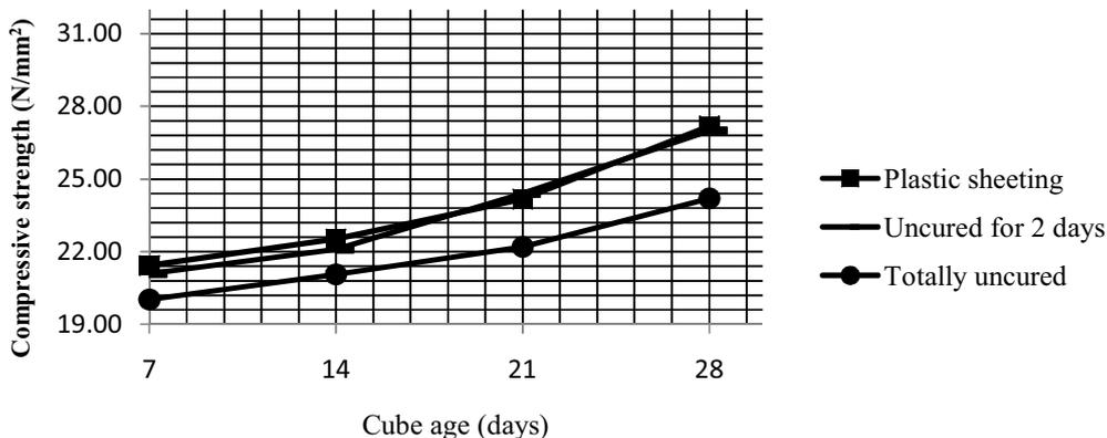
Figure 3: Variation of compressive strength with curing methods.
