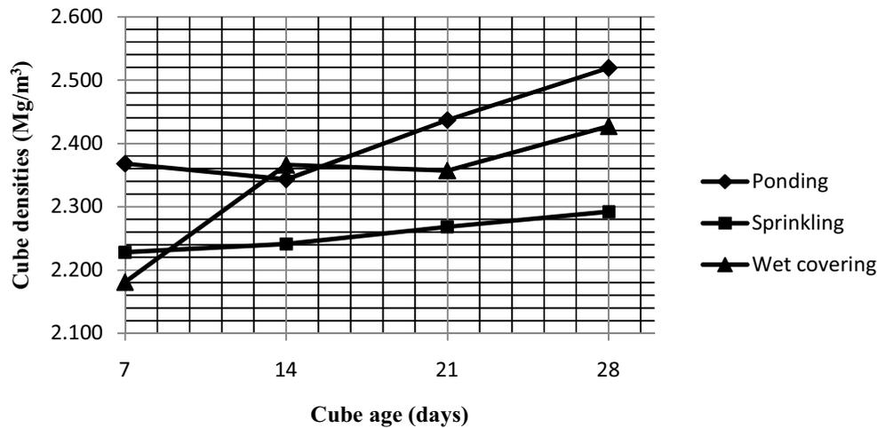
Figure 4: Variation of cube densities with curing methods and age.
