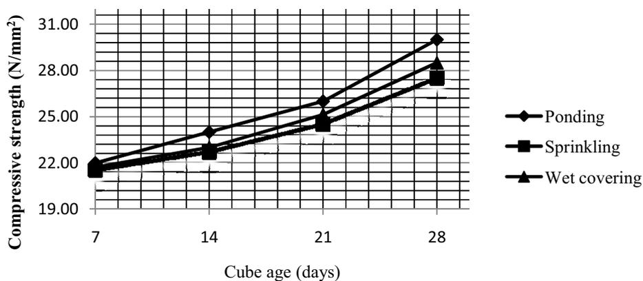
Figure 2: Variation of compressive strength with curing methods.
