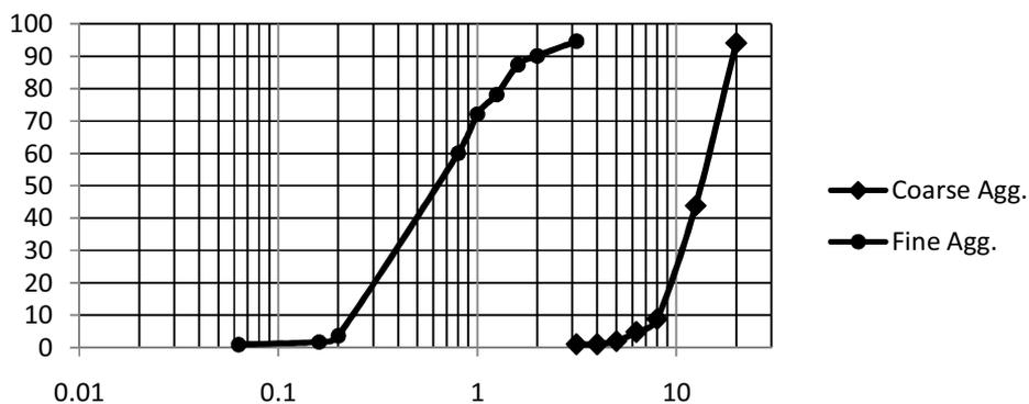
Figure 1: Particle Size Distribution for fine and coarse aggregates (sand and gravel).
