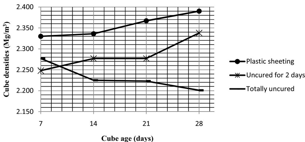
Figure 5: Variation of cube densities with curing methods and age.
