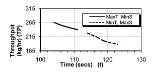
Figure 9: The effect of recycling time on the throughput of the machine under the influence of screw speed (rpm) and torque. Decrease in screw speed and increase in torque while maintaining a constant temperature results to a plot of increase in throughput with corresponding decrease in recycling time. This shows that dependence of the efficiency could be examined as a function of time.
