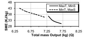
Figure 4: The effect of mass conc. on the SME under the influence of screw speed and torque. By varying the screw speed and torque while maintaining a constant temperature, a plot of the drop in SME with increasing mass concentration is generated and the dependence of the drop in weight could be examined as a function of time.
