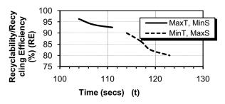
Figure 8: The effect of recycling time on the efficiency of the machine under the influence of screw speed (rpm) and torque. Decreasing screw speed and increasing the torque while maintaining a constant temperature results to a plot of increase in efficiency with corresponding decrease in recycling time. This shows that dependence of the efficiency could be examined as a function of time.
