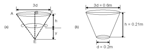
Figure 3: Figure 3 (a) & (b): Frustum of a cone for the hopper.
