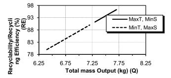
Figure 5: The effect of mass conc. on the efficiency of the machine under the influence of screw speed and torque. Decrease in screw speed and increase in torque while maintaining a constant temperature results to a plot of increase in efficiency with corresponding increase in mass concentration.
