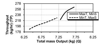
Figure 6: The effect of mass conc. on the throughput of the machine under the influence of screw speed and torque. Decrease in screw speed and increase in torque while maintaining a constant temperature results to a plot of increase in throughput with corresponding increase in mass concentration.
