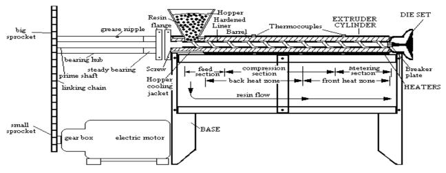
Figure 1: Sectional view of the recycling machine.
