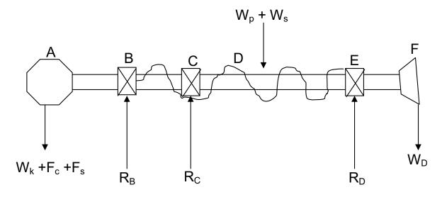
Figure 2: Free body diagram of the screw conveyor unit.
