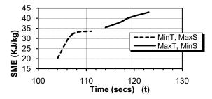
Figure 7: The effect of mass conc. on the SME of the machine under the influence of screw speed (rpm) and torque. Decrease in screw speed and increase in torque while maintaining a constant temperature results to a plot of decrease in SME with corresponding increase in mass concentration.
