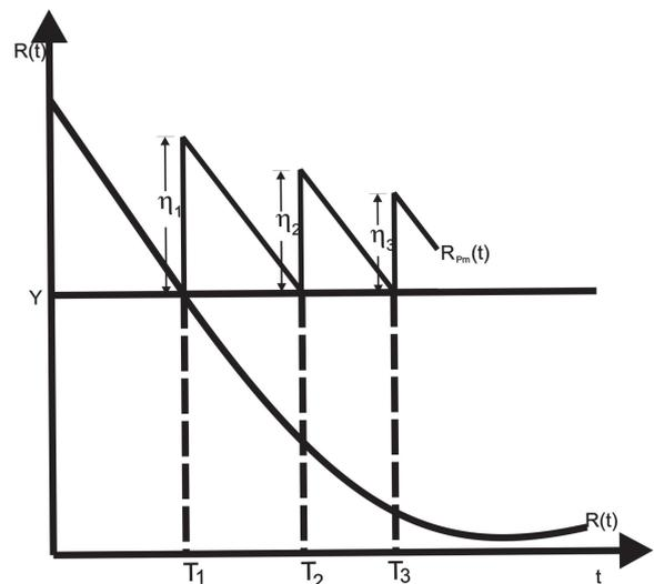
Figure 3: Effect of preventive maintenance on centrifugal pumps
