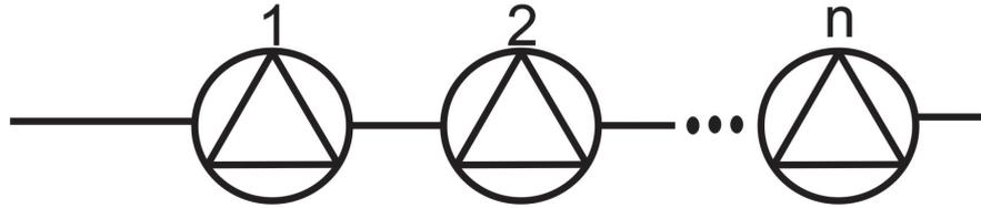
Figure 1: Reliability diagram for centrifugal pumps in series.
