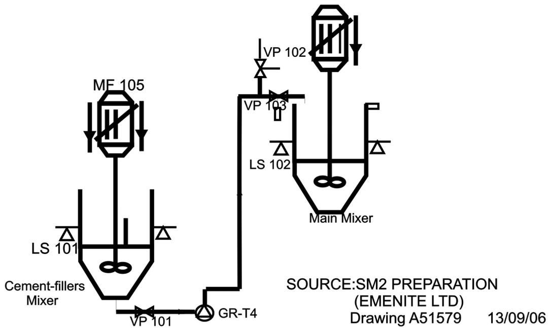
Figure 4: Sketch showing centrifugal pump GR-T4.
