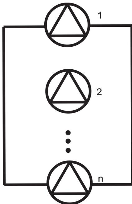
Figure 2: Reliability diagram for centrifugal pumps in parallel.
