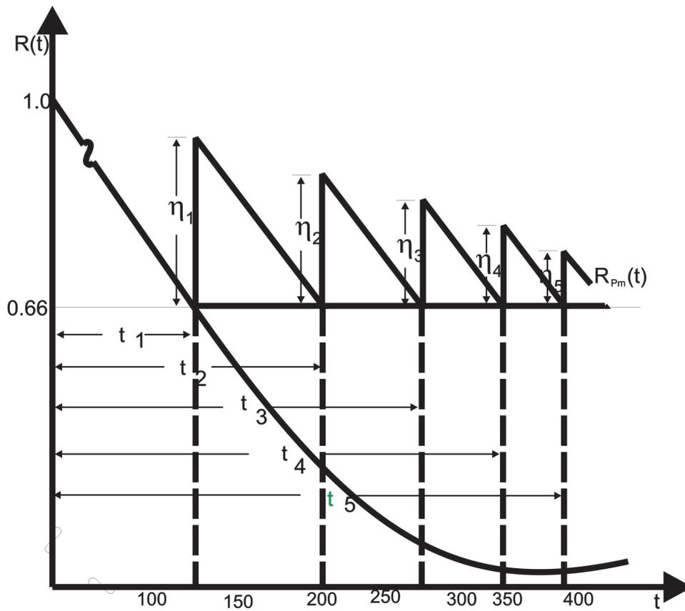
Figure 5: Centrifugal pump preventive maintenance scheduling deterioration and improvement in reliability.
