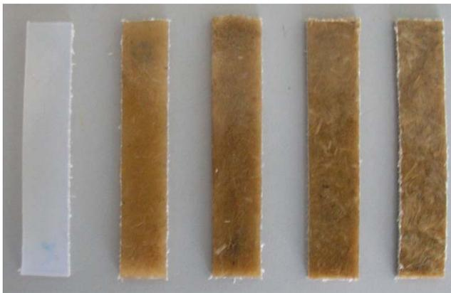
Figure 1: Impact testing specimens of Ukam plant fibre reinforced specimens.
