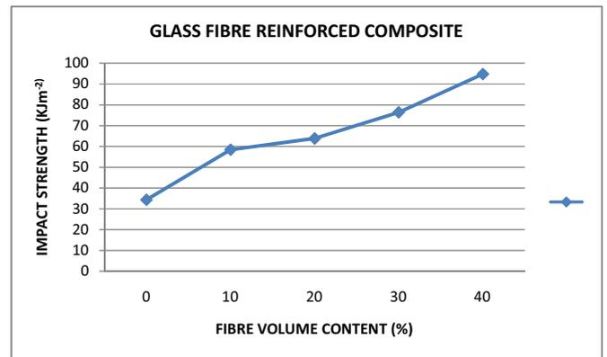
Figure 6: Graph of Impact Strength against Fibre volume content for a Glass fibre reinforced composite.
