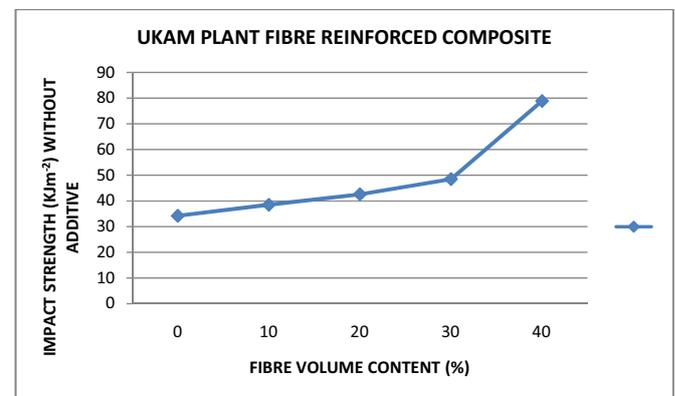
Figure 8: Graph of Impact Strength against Fibre volume content for Ukam plant fibre reinforced composite without additives.
