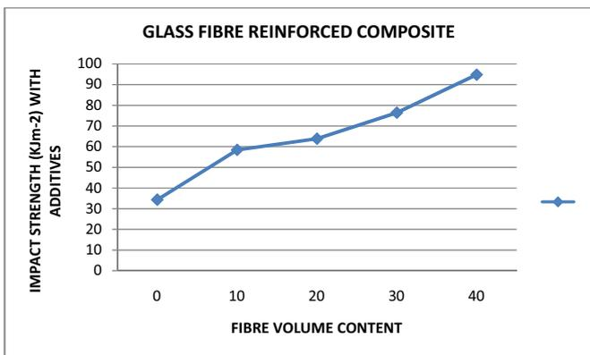
Figure 9: Graph of Impact Strength against Fibre volume content for Glass fibre reinforced composite with additives.
