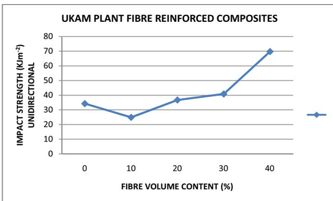
Figure 14: Graph of Impact Strength against Fibre volume content for a unidirectional Ukam plant fibre reinforced composite.
