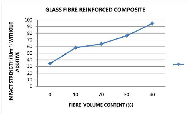
Figure 10: Graph of Impact Strength against Fibre volume content for Glass fibre reinforced composite without additives.
