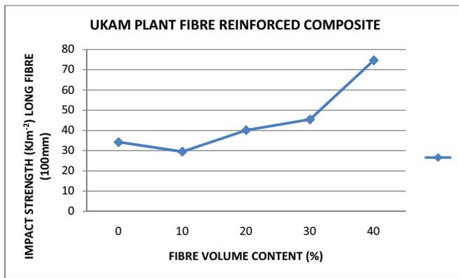
Figure 12: Graph of Impact Strength against Fibre volume content for Long Ukam plant fibre reinforced composite.
