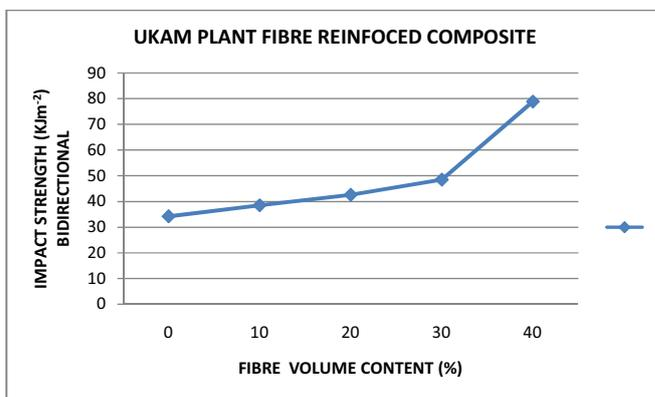
Figure 13: Graph of Impact Strength against Fibre volume content for a bi-directional Ukam plant fibre reinforced composite.
