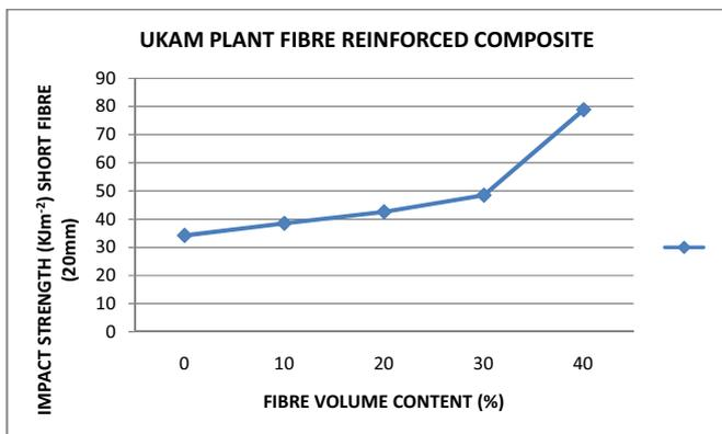
Figure 11: Graph of Impact Strength against Fibre volume content for Short Ukam plant fibre reinforced composite.
