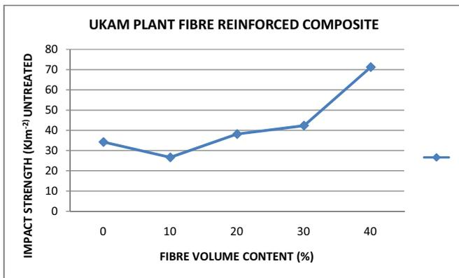
Figure 5: Graph of Impact Strength against Fibre volume content for an untreated Ukam plant fibre reinforced composite.
