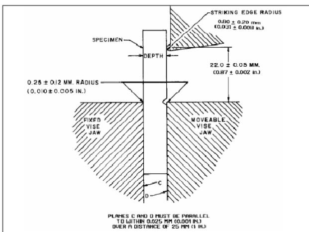
Figure 3: Relation of Vise, Specimen and Striking Edge to Each Other for Izod Test Method A in ASTM D256.
