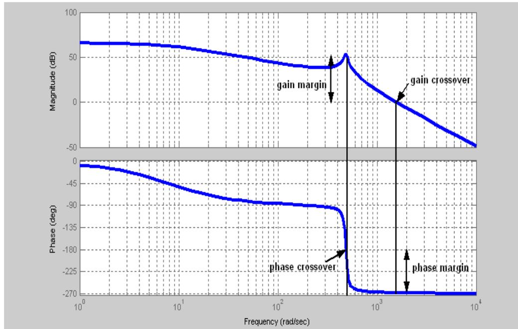
Figure 5: Open loop frequency response of var compensator at no-load operating condition ( $i_{qo} = 0$ ).
