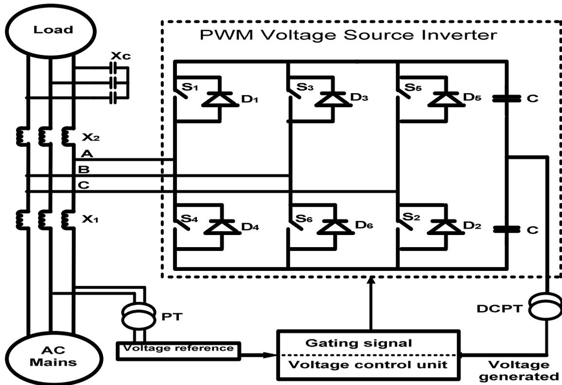
Figure 1: Solid-state var compensator configuration.
