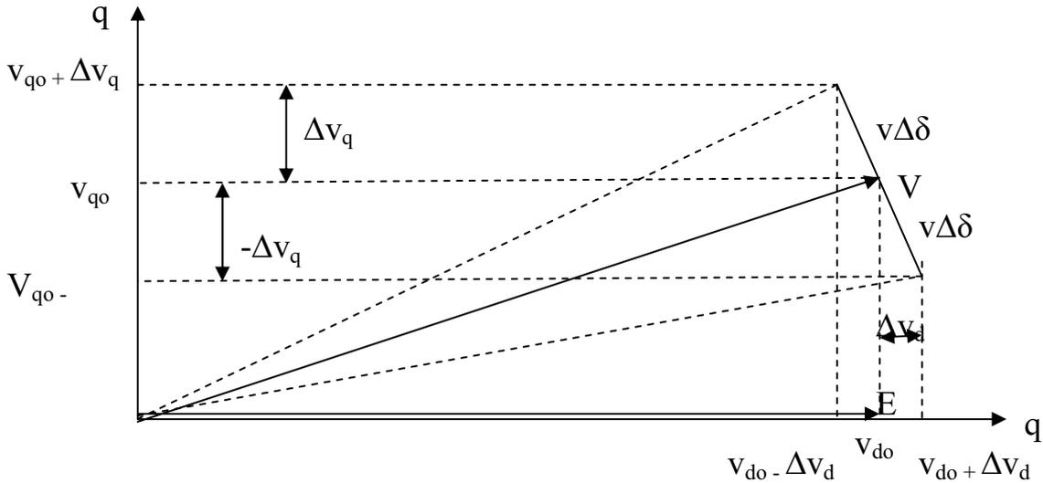
Figure 3: Phasor diagram of the perturbed system.
