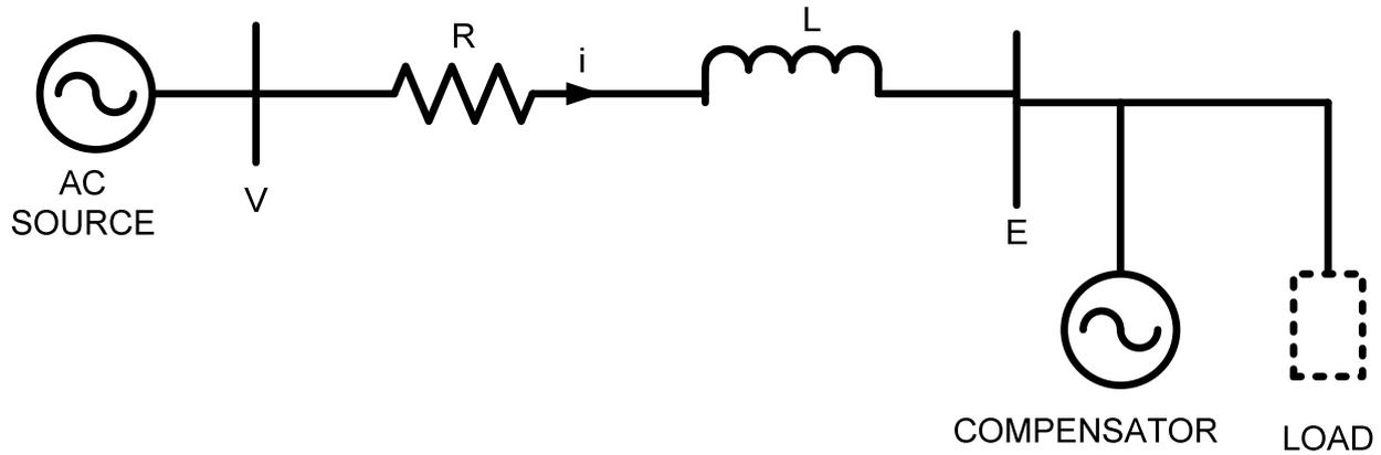
Figure 2: Equivalent circuit per phase of var compensator.  $V$  = Line-to-neutral voltage of the ac mains.  $E$  = Fundamental component of the inverter phase-to-neutral ac voltage.  $i$  = ac current.  $R$  = Losses of the system lumped.  $L$  = Line inductor.
