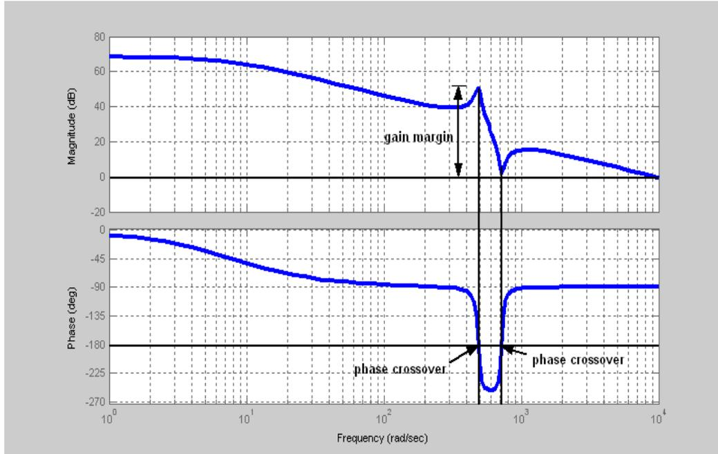
Figure 4: Open loop frequency response of var compensator at rated operating condition ( $i_{qo} = 1$  p.u.).
