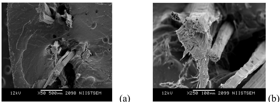
Figure 4: Micrographs of (a)BSF-NR Composite and (b) BBF-NR Composite.
