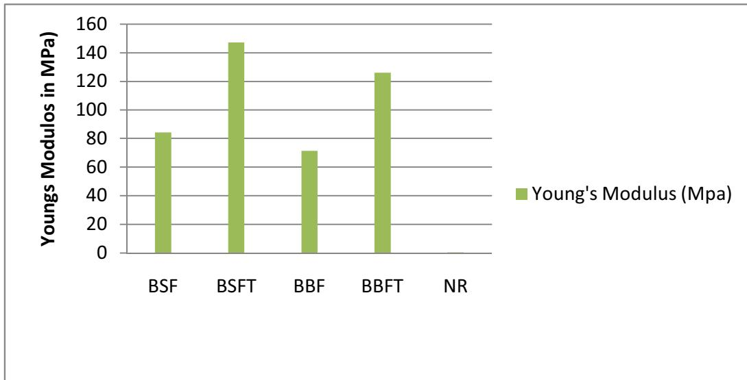
Figure 3: Youngs Modulus properties of untreated and treated banana stem, banana bunch and unreinforced natural rubber(NR) composites.
