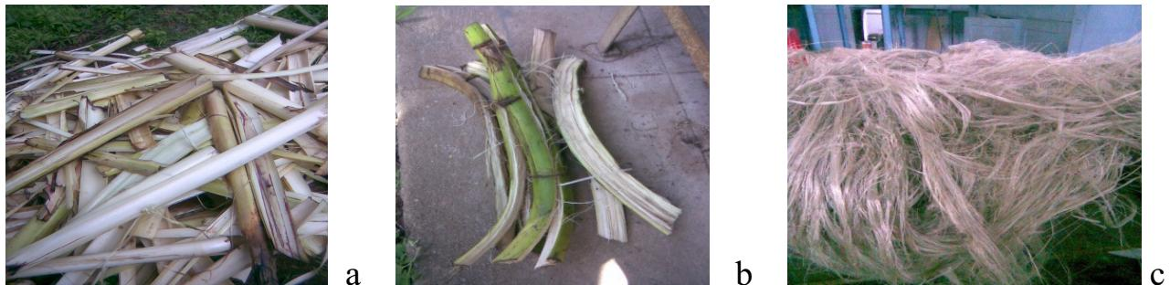
Figure 1: (a) Raw BSF, (b) Raw BBF and (c) extracted BSF samples.
