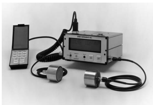
Figure 1: Left: UPV tester. Right: Schematic of UPV apparatus.
