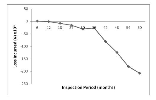
Figure 9: Expected Savings obtained from Inspection frequency of 6 Months when the Manhours spent on Repair Jobs are Less 60% of Workings Hours per Day.
