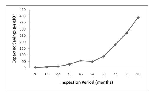
Figure 7: Expected Savings obtained from Inspection frequency of 9 months.
