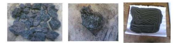
(a) Silicon carbide abrasives (b) An enlarged abrasive chuck (c) Silicon carbide abrasive grains Figure 1. A Sample of produced silicon carbide abrasives and abrasive grains
