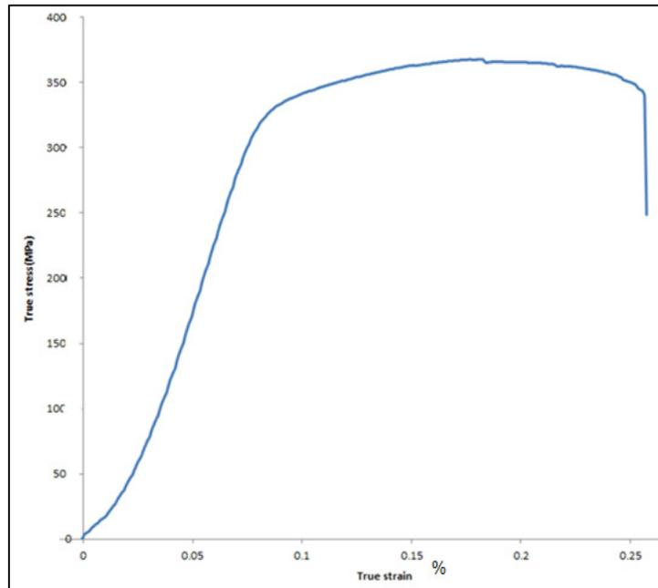
Figure 4: True stress Vs strain curve of as-cast, solution-treated Ti-5Mo-4Nb-2Sn alloy produced for biomedical application.
