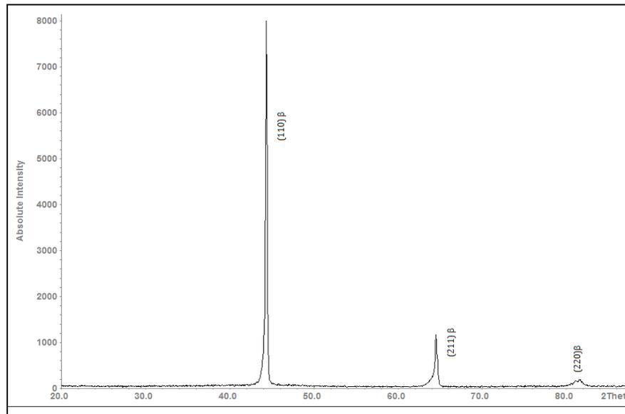
Fig. 2: X-ray diffraction profile of as cast, solution-treated Ti-5Mo-4Nb-2Sn alloy produced for biomedical application
