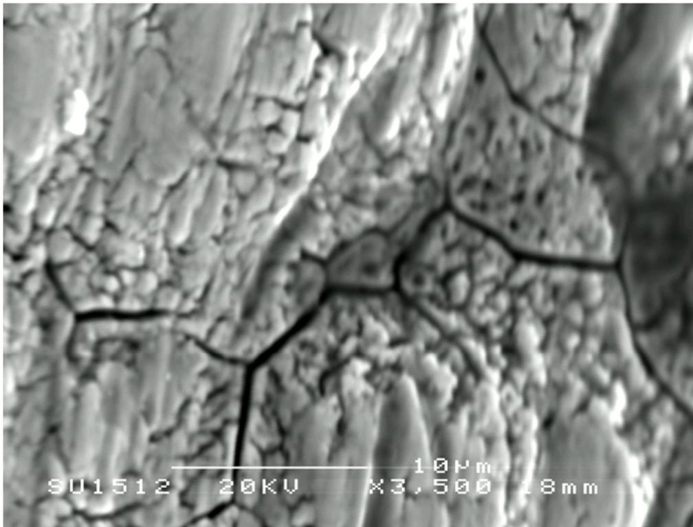
Fig. 3: SEM microstructure of as cast, solution-treated Ti-5Mo-4Nb-2Sn alloy produced for biomedical application
