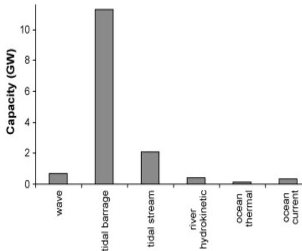
Figure 7: Projected Contributions of various Hydrokinetic Technologies by 2015 (Source: [7])
