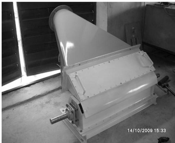
*Fig. 13: Crossflow Turbine developed by NASENI*
