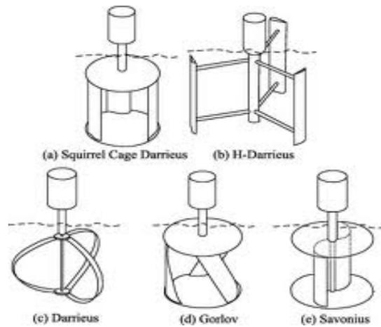
Figure 4: Vertical axis hydrokinetic rotors (Source: [10]).
