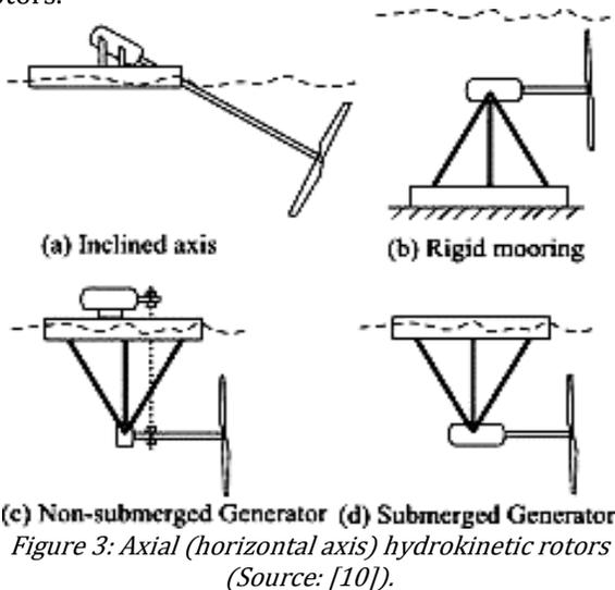
Figure 3: Axial (horizontal axis) hydrokinetic rotors (Source: [10]).
