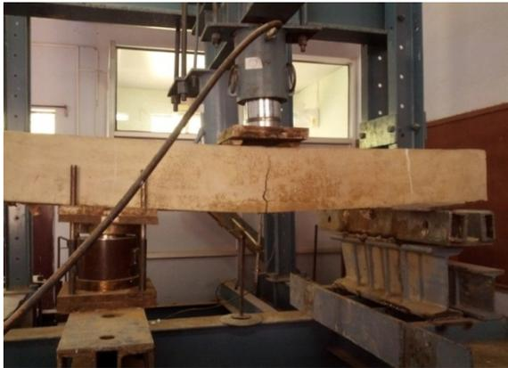
Plate 1: Typical four-point loading set up for the tested samples (control and strengthened)
