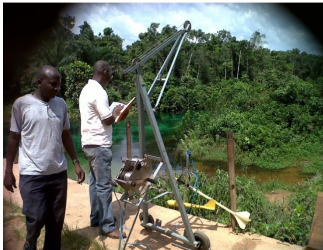
Figure 5: Measuring flow using the Current Meter method.
