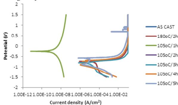
Figure 2: Linear polarization of thermally pre-aged Al-Si-Mg alloy at 105°C in 3.5%NaCl solution at 298K.
