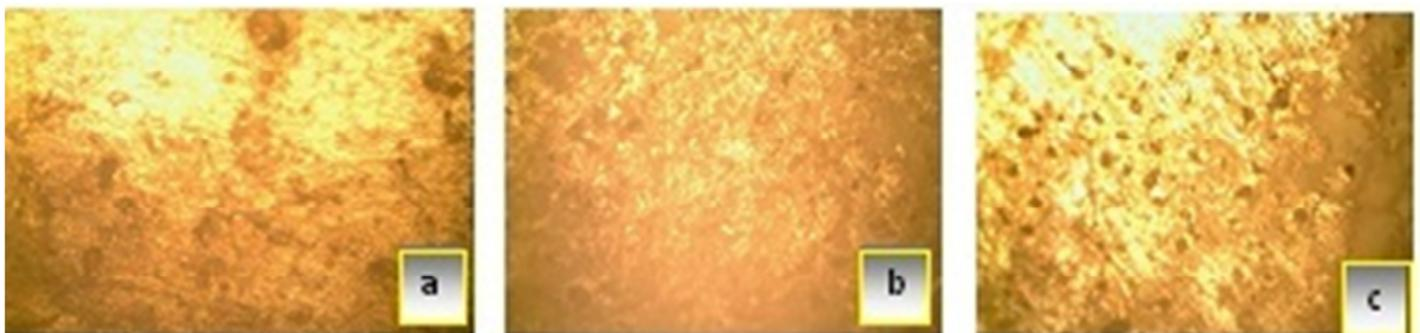
Plate II: OPM of (a.) as cast in the as corroded at 20<sup>th</sup> day (b.) as-corroded at 30<sup>th</sup> day (c.) as-corroded at 40<sup>th</sup> day.
