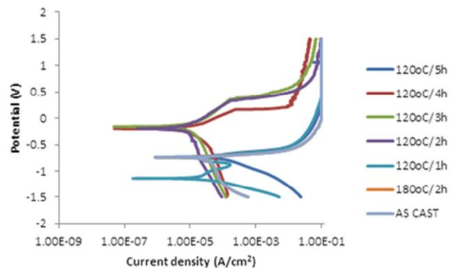
Figure 3: Linear polarization of thermally pre-aged Al-Si-Mg alloy at 120°C in 3.5%NaCl solution at 298K.
