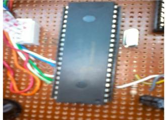
Figure 9: Photo view of the PIC16F877A mounted on connector socket with external 8MHz crystal
