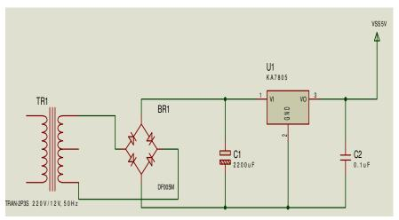
Figure 4: Power supply unit designed on Proteus 8
