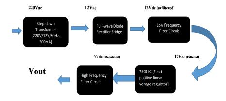
Figure 3: Block diagram of power supply unit
