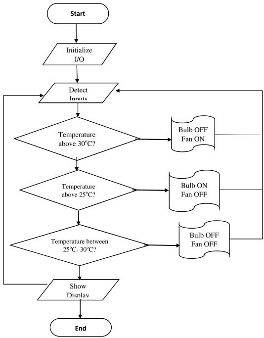
Figure 8. Flow Chart Programming of the Home Automation System
