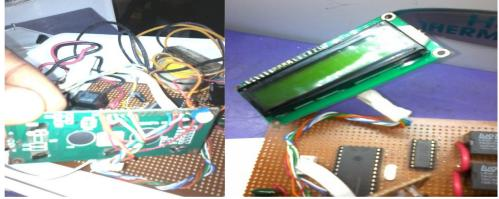
Figure: 10. Liquid Crystal Display Unit showing variable resistor on the back panel
