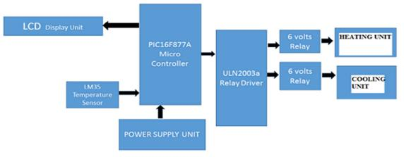
Figure 1: Block Diagram of Temperature Sensor Control System
