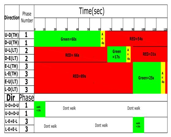
Figure 5: Final signal timing design shown in a timing diagram.
