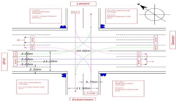
*Figure1: Layout of the intersection at Iyaro showing the number of lanes, width of lanes, and location of traffic signal controllers*
