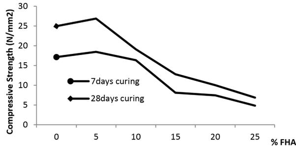
Fig. 1: Compressive Strength of FHAC
