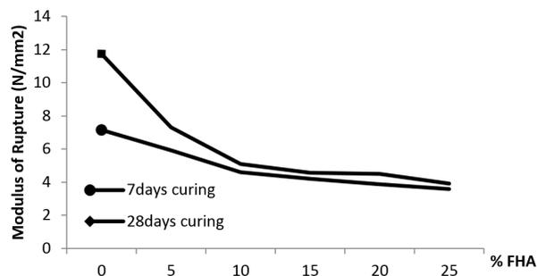
Fig. 2: Flexural Strength of FHAC
