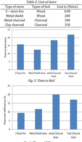
Fig. 6: Thermal Efficiency
