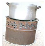
Figure 2: WBT on Metal Shield stove
