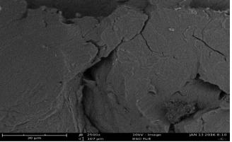
Plate2: SEM microstructure of control samples of Al-6.5%Si-0.35%Mg Alloy
