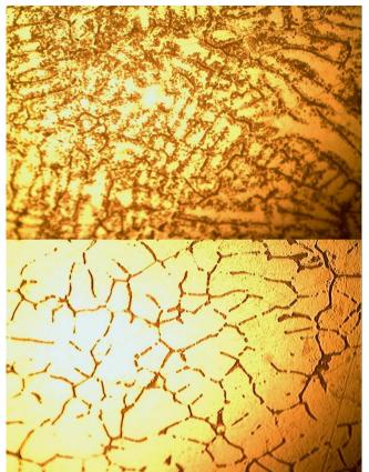
Plates 1: OPM Microstructure of Control and low temperature ageing of 90°C of Al-6.5%Si-0.35%Mg Alloy
