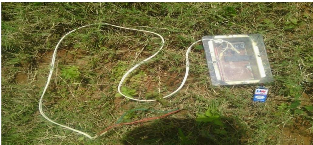
Fig. 4: The Assembled Digital Soil Moisture Meter
