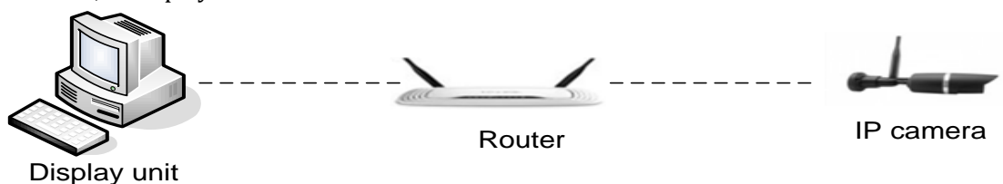
Figure 4: IP Camera connection
