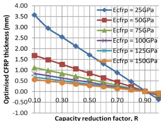
Figure 5: Optimized FRP thickness requirements for various FRP stiffness
