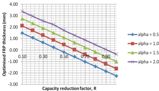
Figure 3: Optimized FRP thickness requirements for various Dead to Live Load Ratio
