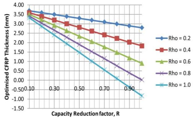
Figure 4: Optimized FRP thickness requirements for various steel reinforcement ratios
