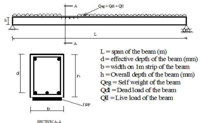
Figure 1: Structural configuration of the beam under investigation
